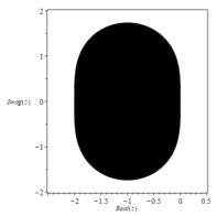
FIGURE 1. The stability region (black shaded) of the second order proposed numerical integration method with the stability interval of (-2.01, 0.01).
