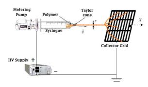
FIGURE 1. Electro-spinning process setup.
