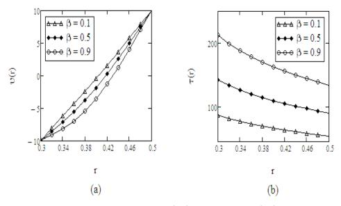
FIGURE 7. Profiles of the velocity v(r,t) and shear stress  $\tau(r,t)$  given by Eqs. (3.18) and (3.22) for  $R_1 = 0.3$ ,  $R_2 = 0.5$ ,  $A_1 = -1$ ,  $A_2 = 1$ , t = 10s,  $\nu = 0.005$ ,  $\mu = 2,916$ ,  $\lambda = 4$  and different values of  $\beta = 0.6$ .
