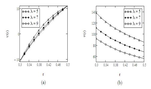
FIGURE 6. Profiles of the velocity v(r,t) and shear stress  $\tau(r,t)$  given by Eqs. (3.18) and (3.22) for  $R_1 = 0.3$ ,  $R_2 = 0.5$ ,  $A_1 = -1$ ,  $A_2 = 1$ , t = 11s,  $\nu = 0.005$ ,  $\mu = 2,916$ ,  $\beta = 0.5$ , and different values of  $\lambda$ .
