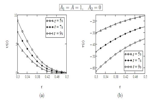
FIGURE 3. Profiles of the velocity v(r,t) and shear stress  $\tau(r,t)$  given by Eqs. (5.3) and (5.4) for  $R_1 = 0.3$ ,  $R_2 = 0.5$ ,  $A_1 = A = 1$ ,  $A_2 = 0$ ,  $\nu = 0.004$ ,  $\mu = 2.916$ ,  $\lambda = 4$ ,  $\beta = 0.5$ , and different values of t.
