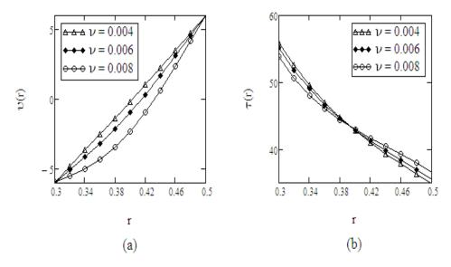
FIGURE 5. Profiles of the velocity v(r,t) and shear stress  $\tau(r,t)$  given by Eqs. (3.18) and (3.22) for  $R_1 = 0.3$ ,  $R_2 = 0.5$ ,  $A_1 = -1$ ,  $A_2 = 1$ , t = 6s,  $\mu = 30$ ,  $\lambda = 2.5$ ,  $\beta = 0.1$ , and different values of  $\nu$ .
