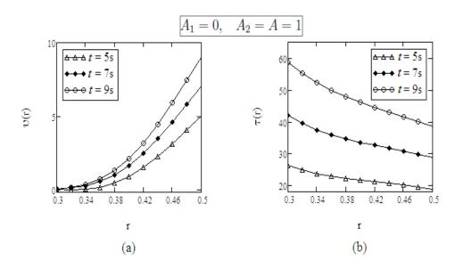
FIGURE 2. Profiles of the velocity v(r,t) and shear stress  $\tau(r,t)$  given by Eqs. (5.1) and (5.2) for  $R_1 = 0.3$ ,  $R_2 = 0.5$ ,  $A_1 = 0$ ,  $A_2 = A = 1$ ,  $\nu = 0.004$ ,  $\mu = 2.916$ ,  $\lambda = 4$ ,  $\beta = 0.5$ , and different values of t.
