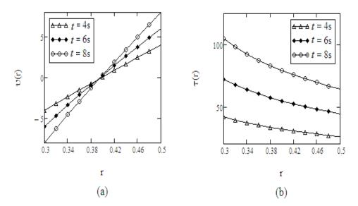
FIGURE 4. Profiles of the velocity v(r,t) and shear stress  $\tau(r,t)$  given by Eqs. (3.18) and (3.22) for  $R_1 = 0.3$ ,  $R_2 = 0.5$ ,  $A_1 = -1$ ,  $A_2 = 1$ ,  $\nu = 0.004$ ,  $\mu = 2.916$ ,  $\lambda = 4$ ,  $\beta = 0.5$ , and different values of t.
