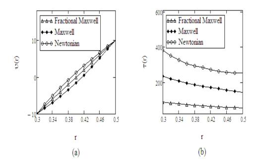
FIGURE 8. Profiles of the velocity v(r,t) and shear stress  $\tau(r,t)$  corresponding to the Newtonian, Maxwell and fractional Maxwell fluids, for  $R_1 = 0.3, R_2 = 0.5, A_1 = -1, A_2 = 1, t = 10s, \nu = 0.004, \mu = 2.916, \lambda = 4$  and  $\beta = 0.1$
