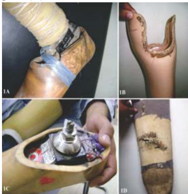
Figure. Damaged prosthetic foot (1A), socket problems (1B), damaged socket adapter (1C), and damaged silicone gelliner (1D).
