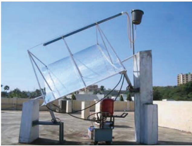
Fig. 10 2 meter x 1.8 meter experimental Solar Parabolic Trough developed at PNEC, that heats the 2.3 liters of Heat Transfer Fluid (HTF) in the central tube to over 300 Co.
