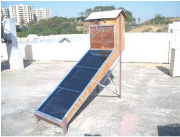
Fig. 12 Two views of a solar drier, used to dry and preserve perishable food
