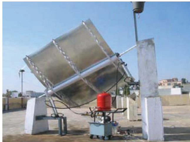
Fig. 10 2 meter x 1.8 meter experimental Solar Parabolic Trough developed at PNEC, that heats the 2.3 liters of Heat Transfer Fluid (HTF) in the central tube to over 300 Co.
