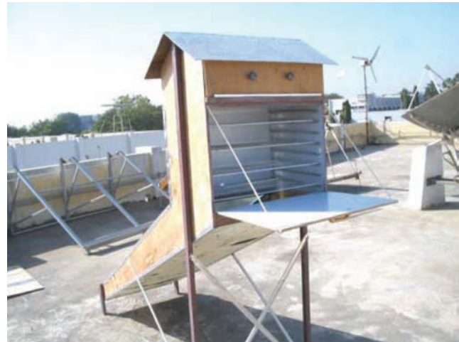
Fig. 12 Two views of a solar drier, used to dry and preserve perishable food
