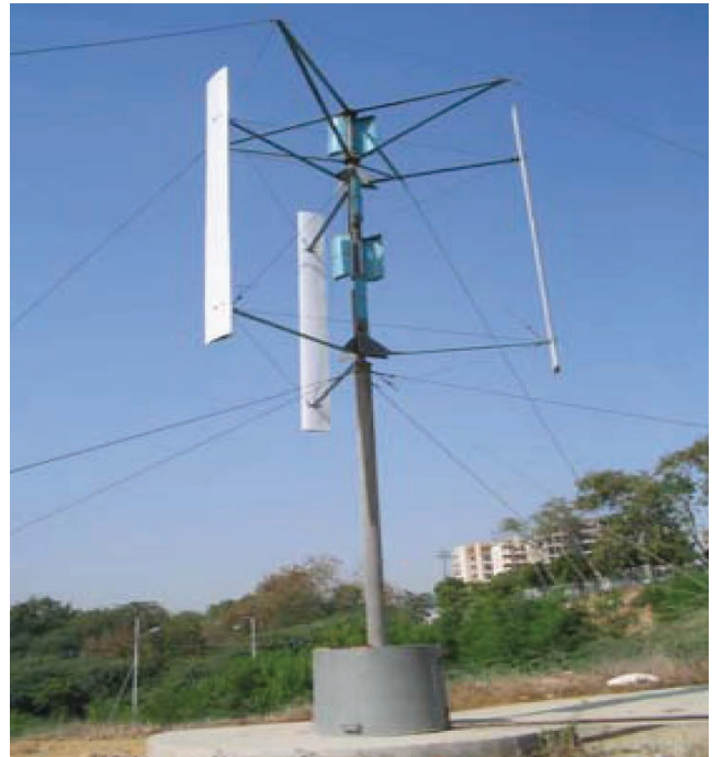
Fig. 3 Three bladed 1000 watt vertical axis wind turbine with a combination of Savonius and Darrieus type blades
