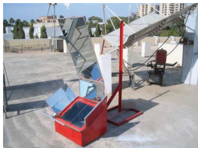
Fig. 15 Box type solar cooker with four additional booster mirrors
