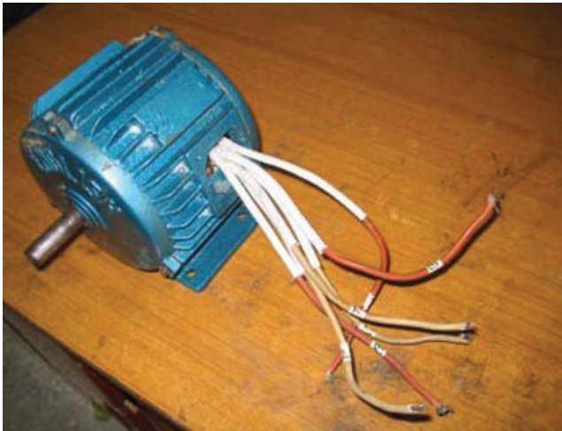
Fig. 9 Wind turbine electric generators of 500 watt and 1500 watt power capacity developed at PNEC.
