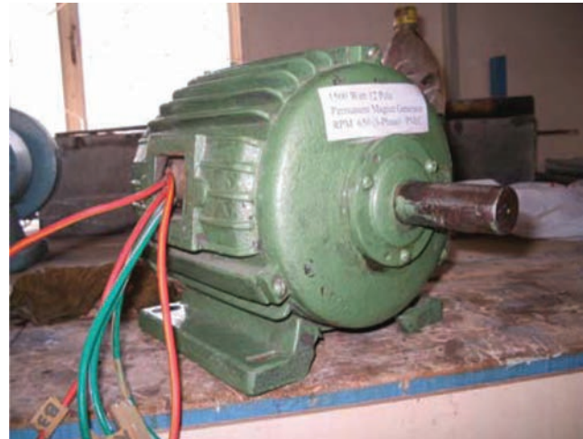
Fig. 9 Wind turbine electric generators of 500 watt and 1500 watt power capacity developed at PNEC.
