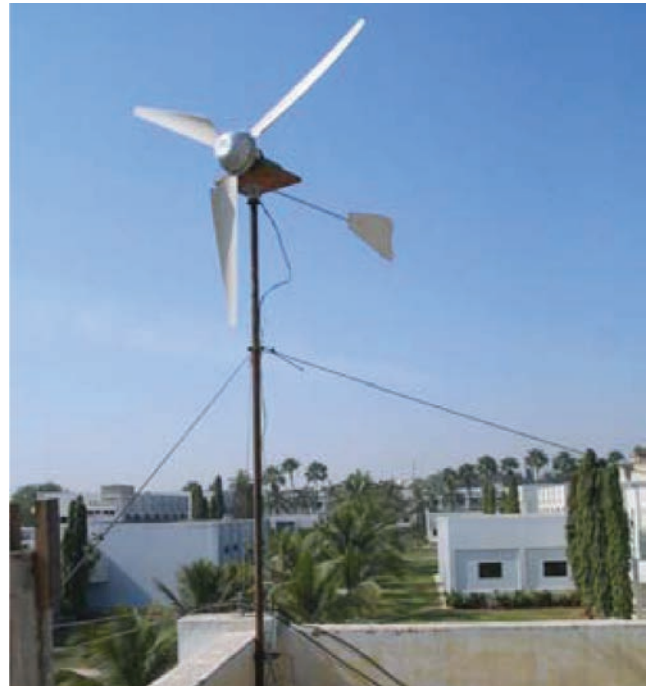
Fig. 7 Three bladed 300 watt horizontal axis wind turbine with PVC blades
