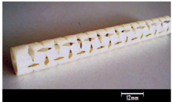
**Figure 11:** Master model (Auxetic airway stent) made of ABS plastic by FDM process
