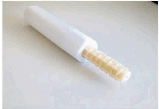
**Figure 7: A tubular template is fixed tightly within TEFLON tube**
