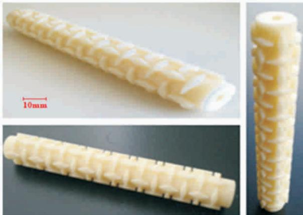
**Figure 6: An antipode-Auxetic template made by ABS plastic**
