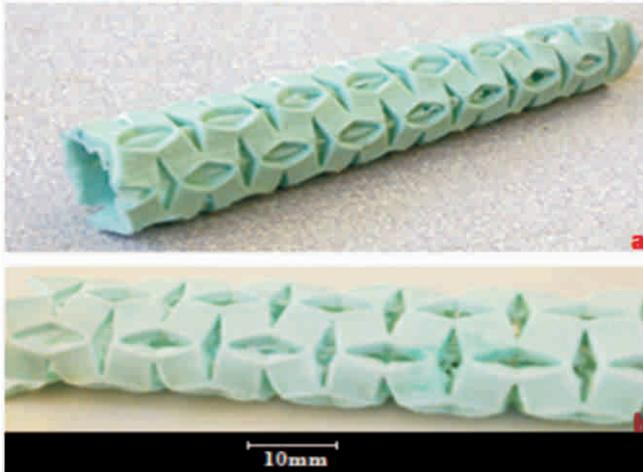
**Figure 9:**(a) Auxetic stent removed from the template with some material intact within the diamond-shaped areas, and (b) material removed by the tweezers
