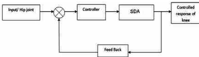
Figure 4: Control System for SDA
