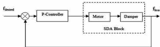
Figure 5: P controller for SDA
