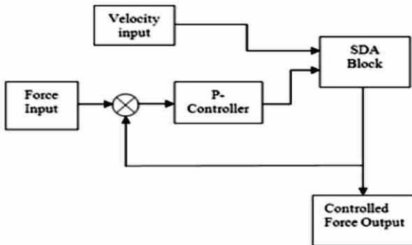
Figure 10: SDA Controller with Velocity Input
