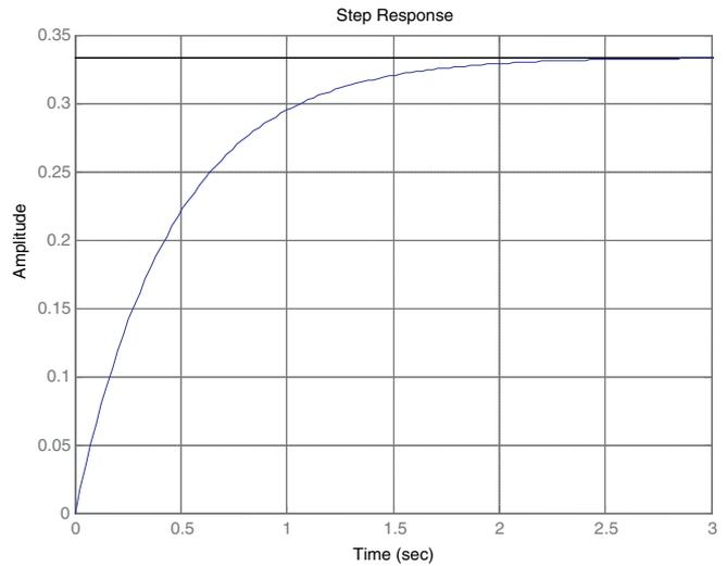
Figure 7: Open Loop Response of SDA
