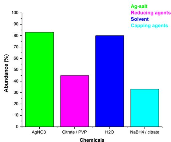
**Fig. 1a: Most frequently employed chemicals for the synthesis of Ag nanoparticles [19].**
