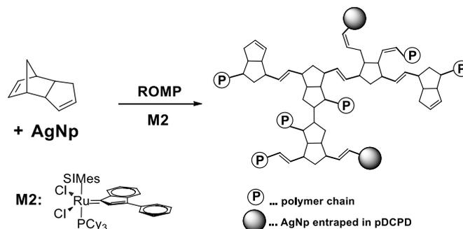
**Fig. 2: Specimen example for ROMP of DCPD in presence of 1w% Oleylamine stabilized silver nanoparticles [19]**
