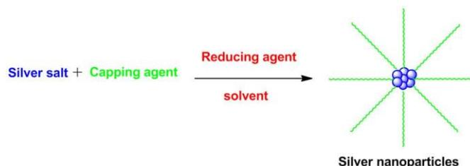
**Scheme 1: The general reaction scheme for the synthesis of silver nanoparticles**
