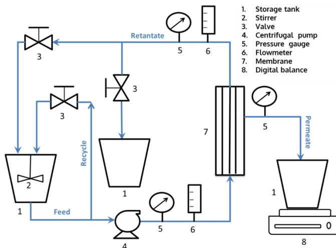
**Fig. 1: Laboratory scale Crossflow microfiltration unit.**
