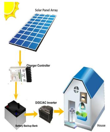
Figure 3. Schematic diagram of proposed off-grid solar photovoltaic system
