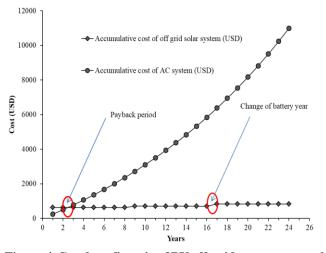
Figure 4. Cost benefit ratio of PV off-grid system on yearly basis
