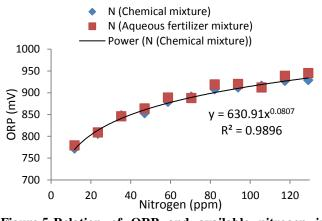
Figure 5. Relation of ORP and available nitrogen in chemical (NO<sub>3</sub><sup>-</sup>, H<sub>3</sub>PO<sub>4</sub>, K<sup>+</sup>) and aqueous fertilizer (NO3<sup>-</sup>, TSP, MOP) mixtures
