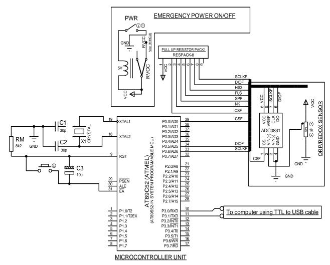
Figure 2. Design of controller for ORP sensor
