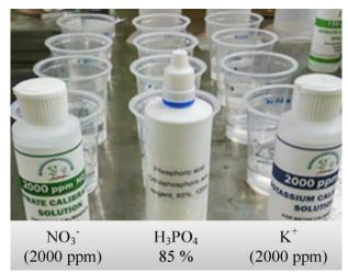
Figure 4. Solutions used for calibration and validation of ORP sensor
