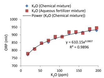
Figure 7. Relation of ORP and K<sub>2</sub>O in chemical (NO<sub>3</sub><sup>-</sup>, H<sub>3</sub>PO<sub>4</sub>, K<sup>+</sup>) and aqueous fertilizer (NO<sub>3</sub><sup>-</sup>, TSP, MOP) mixtures
