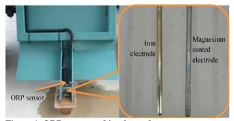
Figure 1. ORP sensor and its electrodes
