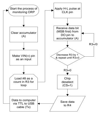
Figure 3. Programing algorithm of getting fertility data from ORP sensor
