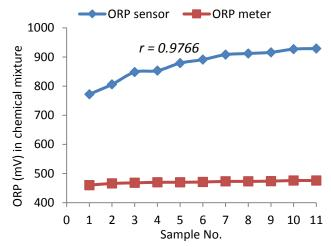
Figure 8. Correlation of ORP sensor values with ORP-200 meter values in chemical (NO<sub>3</sub><sup>-</sup>, H<sub>3</sub>PO<sub>4</sub>, K<sup>+</sup>) mixture
