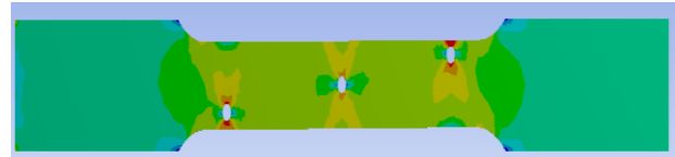
Fig 20: 0.1-inch three diagonally distributed specimen under stress
