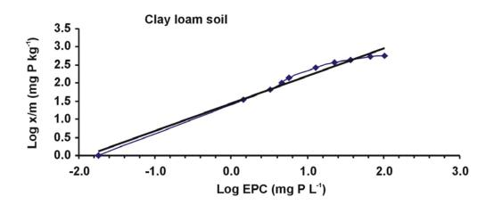
this study maximum buffering capacity (159.92 mg P kg<sup>-1</sup>) was observed in clay loam soil followed by loam and sandy loam soils (Table 3). The values of exponent (1/n) represent the extent of adsorption and expressed as mg P kg<sup>-1</sup> soil. In this study these values ranged from 0.579 to 0.718 L kg<sup>-1</sup>. Similar values of exponent (1/n) were observed by a number of other researchers (Zhou and Li, 2001., Hussain *et al.*, 2006).
