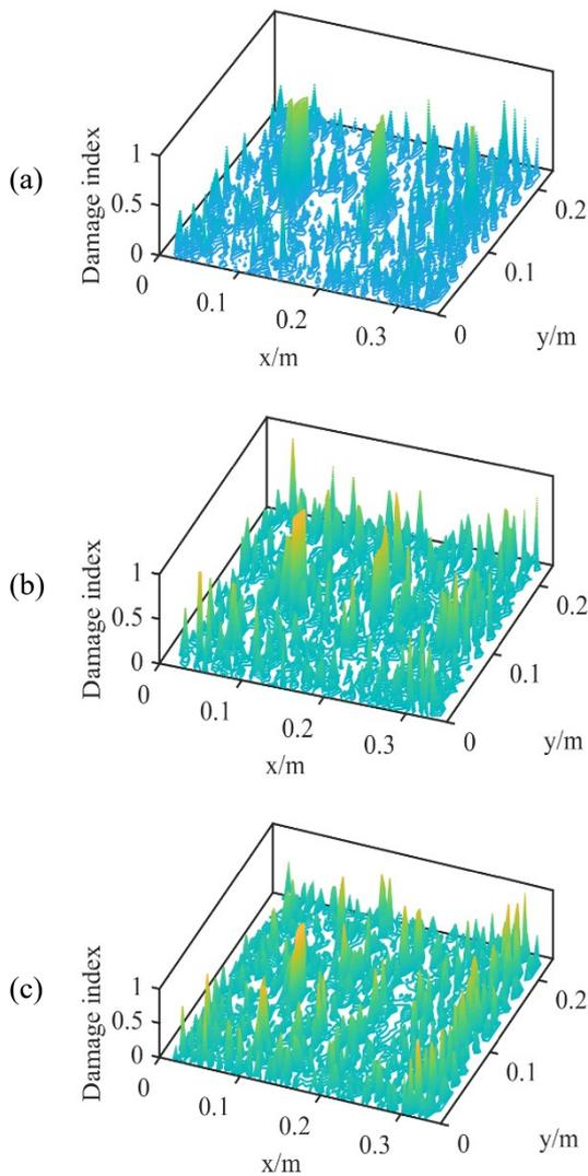
**Fig. 5:** Damage indices with 0.1% noise for damage scenario 1; (a) 11.2% severity, (b) 7.2% severity, (c) 3.5% severity
