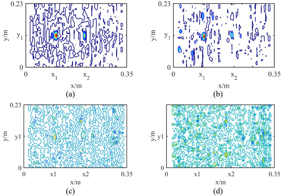
**Fig. 9:** Estimated damage indices for Scenario 1 with noise levels of: (a)  $5 \times 10^{-4}$ , (b)  $1 \times 10^{-3}$ , (c)  $5 \times 10^{-3}$  and (d)  $1 \times 10^{-2}$
