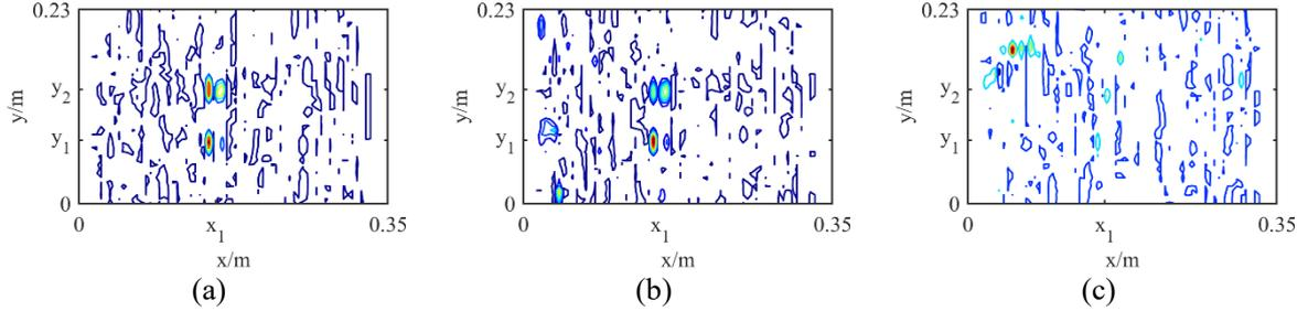
**Fig. 8:** Estimated damage indices after using Bayesian approach for scenario 2: (a) 11.2% severity, (b) 7.2% severity, (c) 3.5% severity
