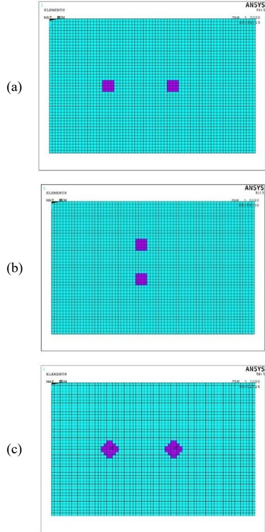
**Fig. 2:** Finite element model of the plate with damage zones: (a) Scenerio 1, (b) Scenerio 2, (c) Scenario 3
