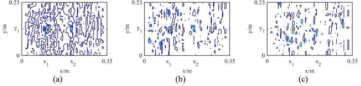
**Fig. 7:** Estimated damage indices after using Bayesian approach for scenario 1: (a) 11.2% severity, (b) 7.2% severity, (c) 3.5% severity
