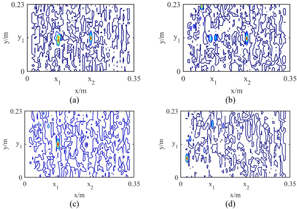
**Fig. 10:** Estimated damage indices for Scenario 3 with noise levels of: (a)  $5 \times 10^{-4}$ , (b)  $1 \times 10^{-3}$ , (c)  $5 \times 10^{-3}$  and (d)  $1 \times 10^{-2}$
