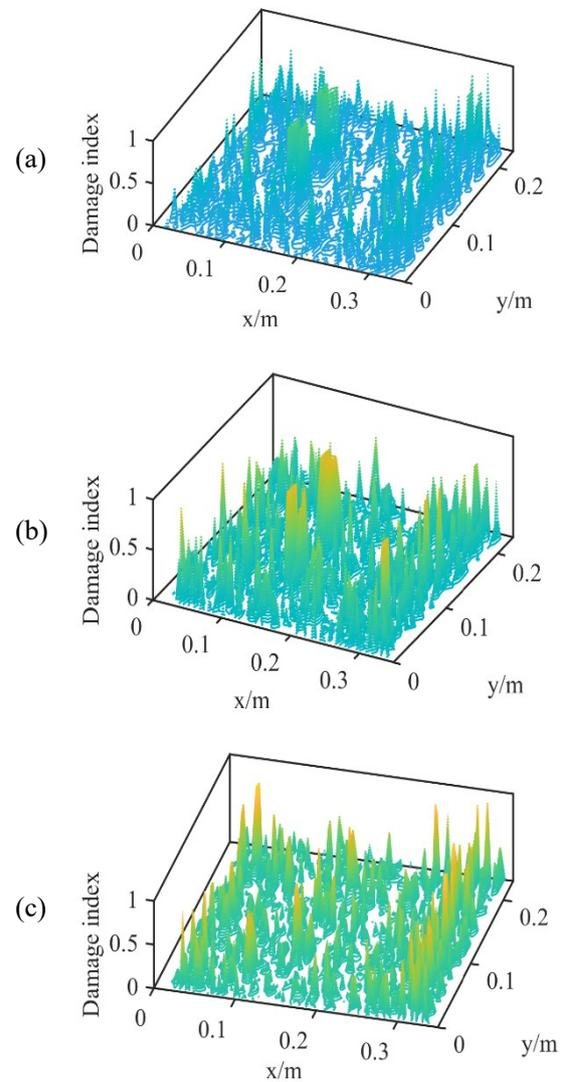
**Fig. 6:** Damage indices with 0.1% noise for damage scenario 2; (a) 11.2% severity, (b) 7.2% severity, (c) 3.5% severity
