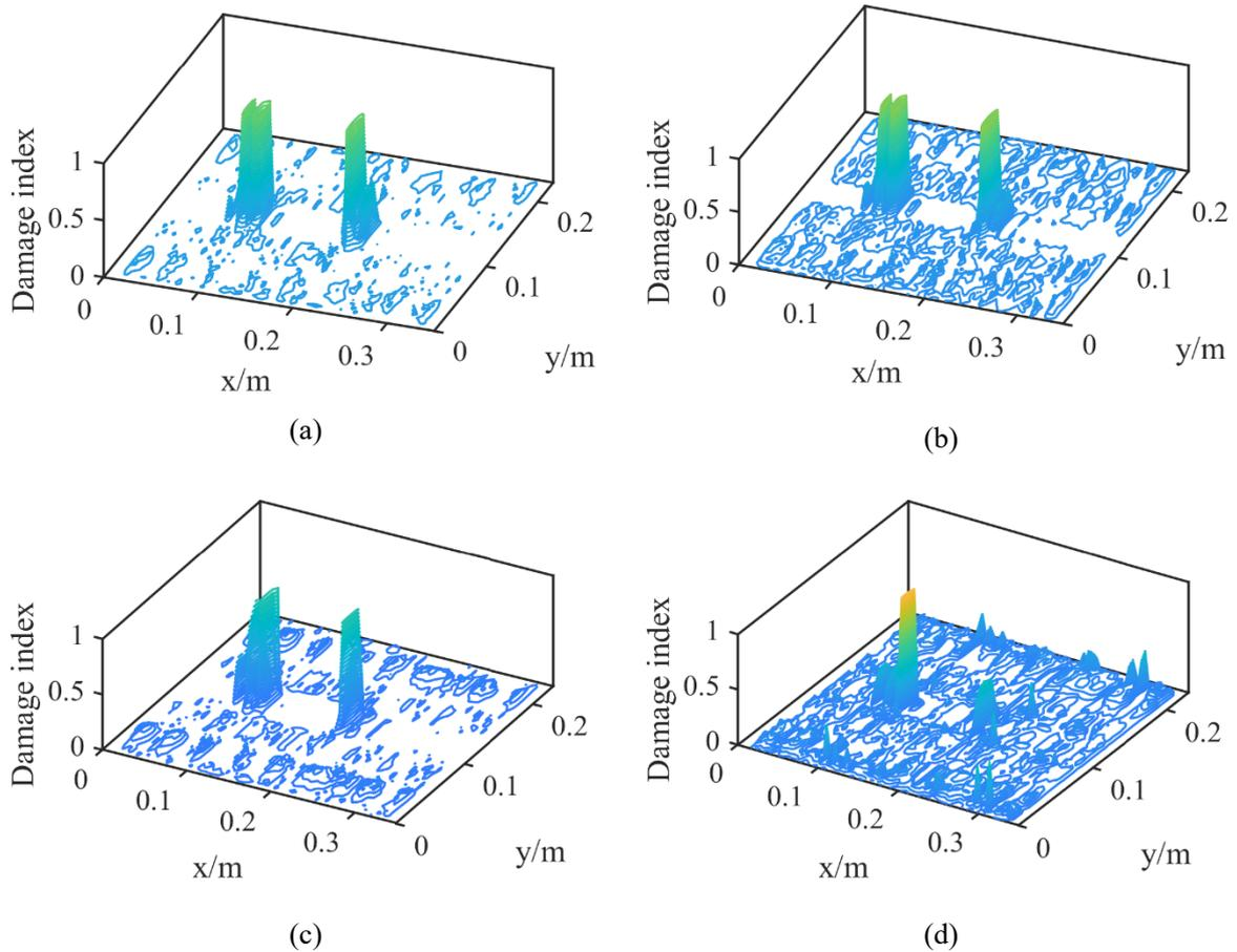
**Fig. 3:** Damage index for different severities of damage scenario 1: (a) 11.2% severity, (b) 7.2% severity, (c) 3.5% severity and (d) 1.7% severity
