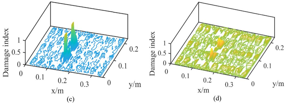
**Fig. 4:** Damage index for different severities of damage scenario 2: (a) 11.2% severity, (b) 7.2% severity, (c) 3.5% severity and (d) 1.7% severity
