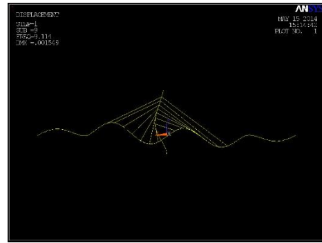
Fig. 12. 9 th mode shape of the Bridge Model under free vibrations
