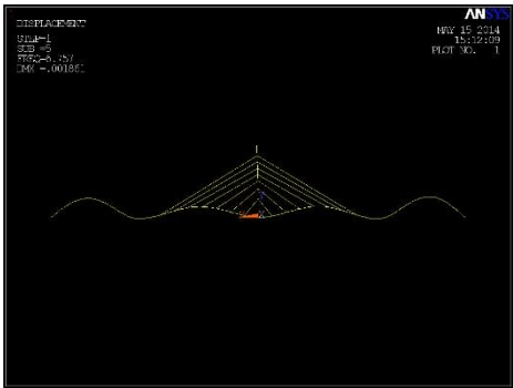
Fig. 8. 5 th mode shape of the Bridge Model under free vibrations
