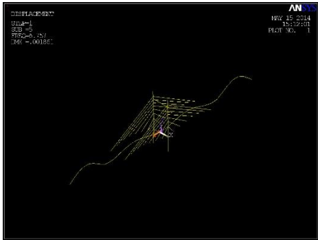
Fig. 7. 4 th mode shape of the Bridge Model under free vibrations
