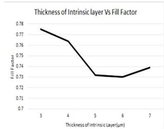
**Figure 8:** Graph between thickness of intrinsic layer and fill factor
