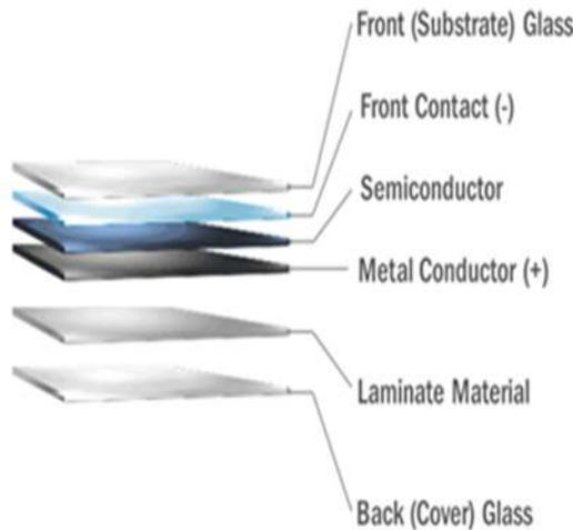
**Figure 2:** Thin film solar cell and its constituent's layers
