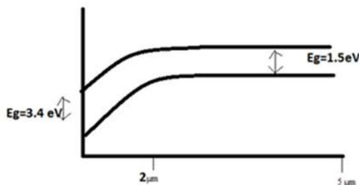
**Figure 4:** Bandgap diagram of Gallium Nitride /polysilicon solar cell
