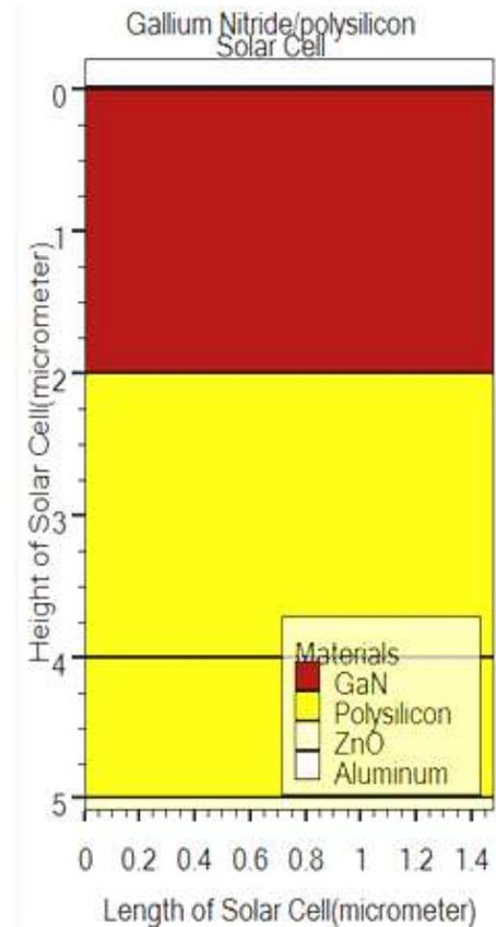
**Figure 3:** Dimensions of proposed Gallium Nitride /Polysilicon Solar Cell
