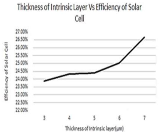
**Figure 9:** Graph between thickness of intrinsic layer and efficiency of solar cell
