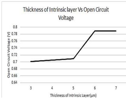
**Figure 6:** Graph between thickness of intrinsic layer and open circuit voltage
