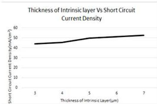
**Figure 7:** Graph between thickness of intrinsic layer and short circuit current density
