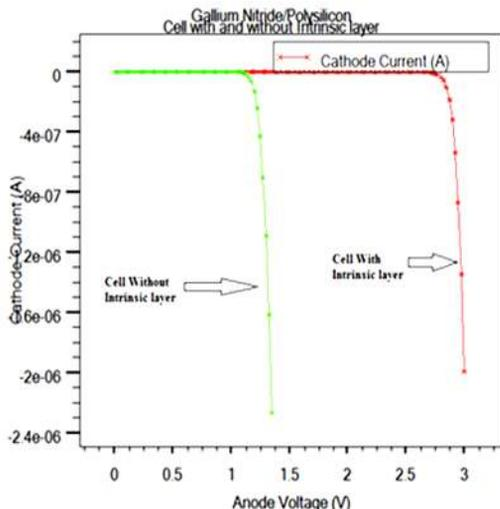
**Figure 5:** Investigation of Gallium Nitride/polysilicon solar cell with and without intrinsic layer
