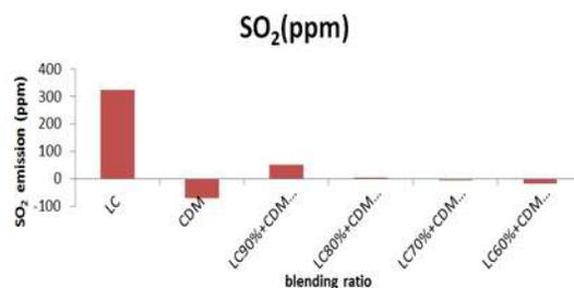
Figure 4: Effect of different blending ratio of coal and Cow dung manure on SO<sub>2</sub> emission
