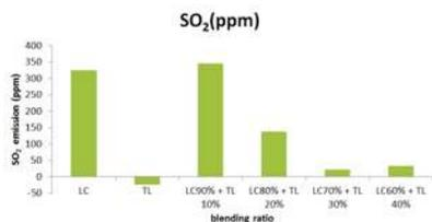
Figure 3: Effect of different blending ratio of coal and tree leaves on SO<sub>2</sub> emission
