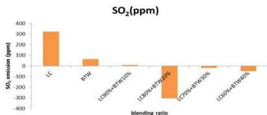
Figure 2: Effect of different blending ratio of coal and banana tree waste on SO<sub>2</sub> emission
