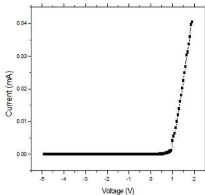
**Figure 3:** The graph between I-V of SiC at T= 320K.
