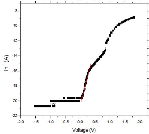
Figure 8: The graph between V and  $\ln(I_s)$  of SiC at T= 360K
