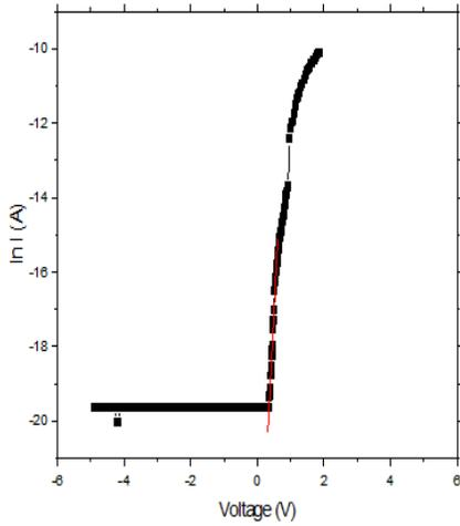
Figure 4: The graph between V and  $\ln(I_s)$  of SiC at T= 320K.
