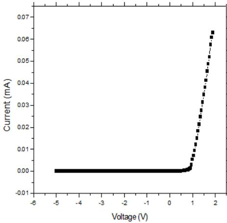
Figure 5: The graph between I-V of SiC at T= 340K.
