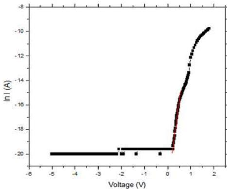
Figure 6: The graph between V and  $\ln(I_s)$  of SiC at T= 340K.
