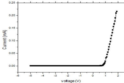
Figure 11: The graph between I-V of SiC at  $T=400K$ .
