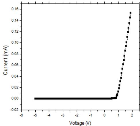
Figure 9: The graph between I-V of SiC at T= 380K
