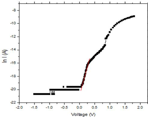
Figure 10: The graph between  $V$  and  $\ln(I_s)$  of SiC at  $T=380K$ .
