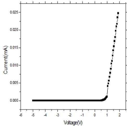
**Figure 1:** The graph between I-V of SiC at T= 295K.
