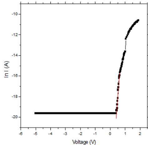
**Figure 2:** The graph between V and ln(I<sub>s</sub>) of SiC at T= 295K
