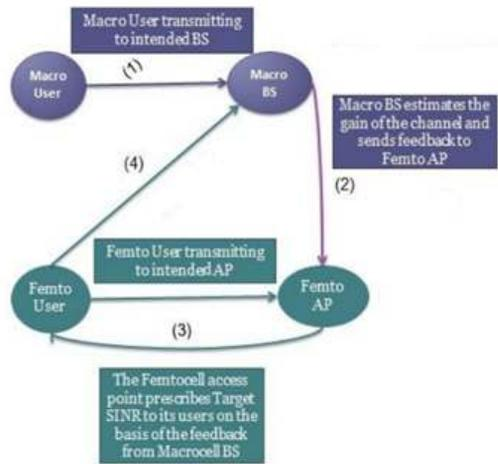
**Figure 2:** Elaboration of Proposed Power Control Scheme
