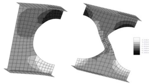
**Figure 6:** Contours for normal traction in longitudinal direction for partitions 1 and 2 (Units: N/m as thickness is included in stress resultant)
