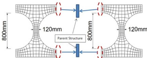
**Figure 4:** Connectivity of partition modules with the parent structure
