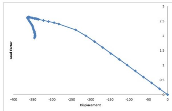
**Figure 7:** Displacement at mid-span in the cellular beam
