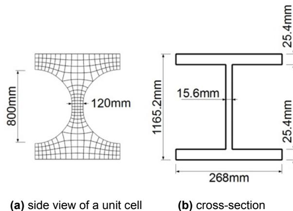
Figure 2: Side elevation of a unit cell and cross-section of the cellular beam
