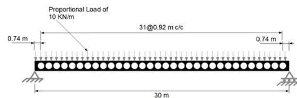
Figure 1: Side elevation of the cellular beam
