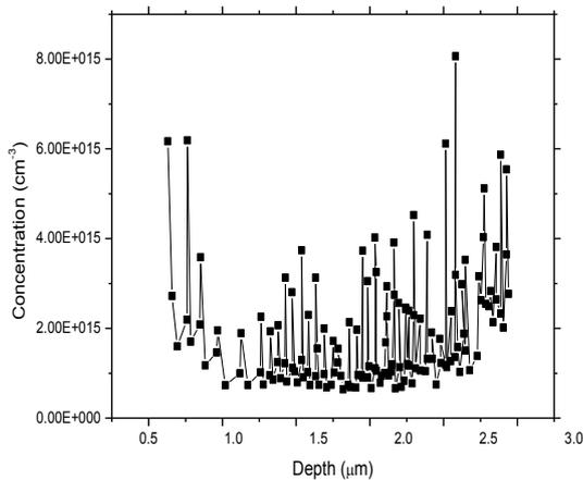
Figure 11: Depth profile of InGaN at temperature 280K .
