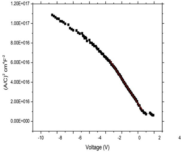
Figure 4: The graph between V and  $(A/C)^2$  of InGaN at T=260K.
