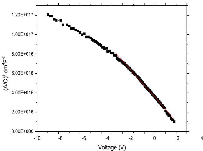
Figure 6: The graph between V and  $(A/C)^2$  of InGaN at T=220K.
