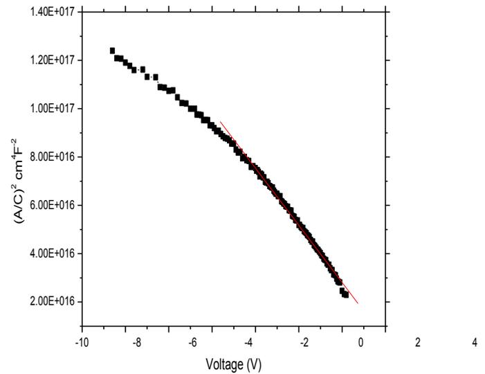
Figure 8: The graph between V and  $(A/C)^2$  of InGaN at T=200K.
