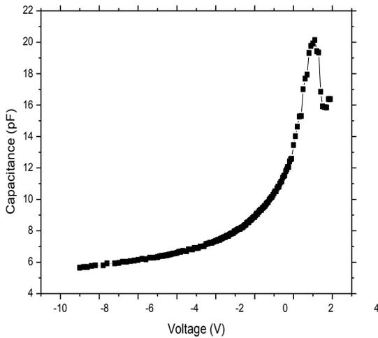
Figure 5: The graph between C-V of InGaN at T=220K .
