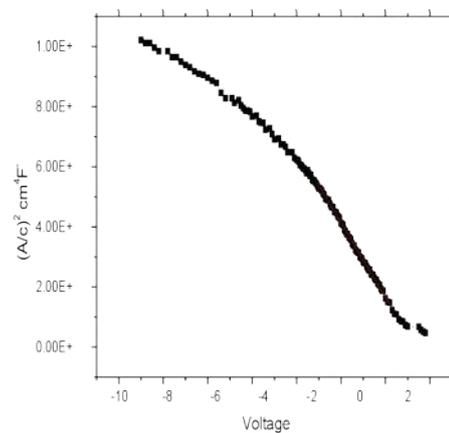
Figure 2: The graph between V and (A/C)<sup>2</sup> of InGaN at T=280K.
