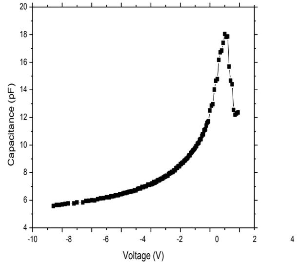
Figure 7: The graph between C-V of InGaN at T=200K
