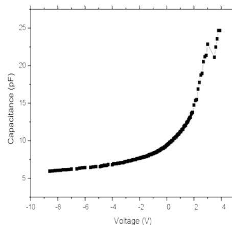
Figure 3: The graph between C-V of InGaN at T=260K
