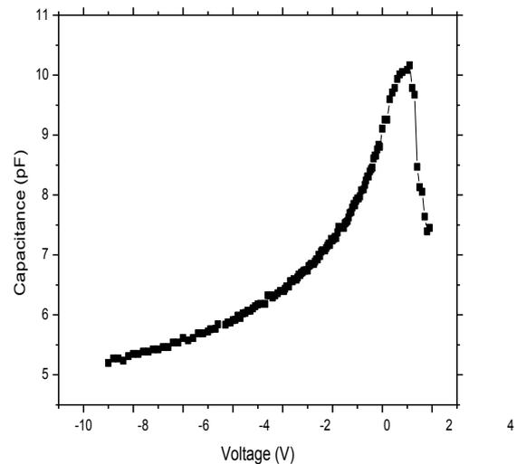
Figure 9: The graph between C-V of InGaN at T=167K .
