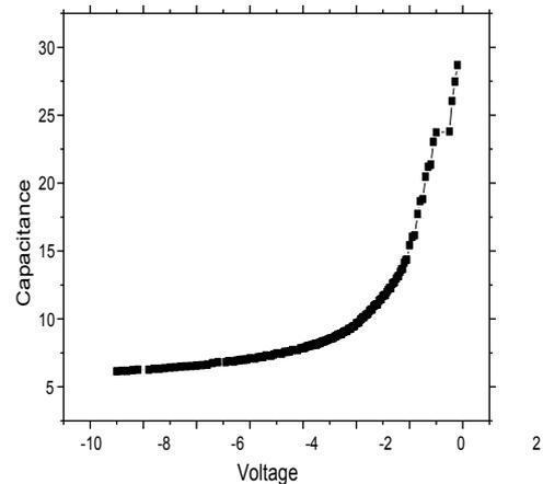
Figure 1: The graph between C-V of InGaN at T=280K.
