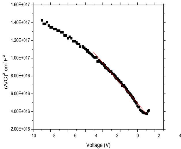
Figure 10: The graph between  $V$  and  $(A/C)^2$  of InGaN at  $T=167K$ .
