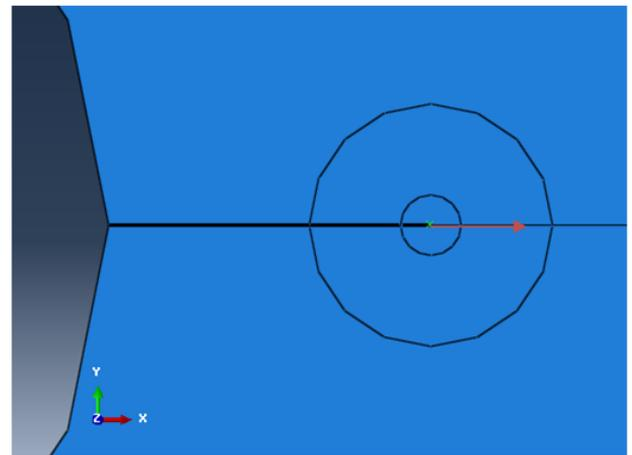
Fig. 7. Close-up with assigned seam and crack propagation direction
