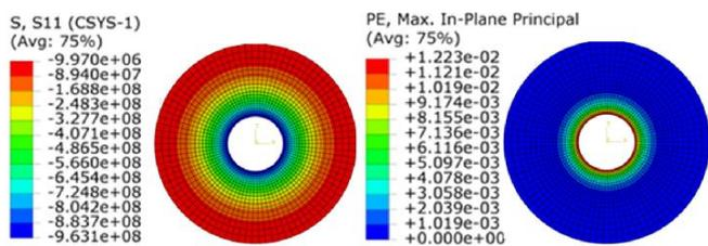
Fig. 11 (a) Hoop stress (b) Plasticity for 1000 MPa internal pressure
