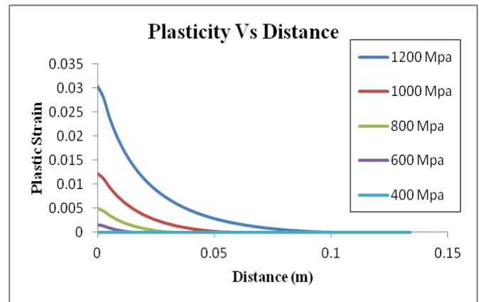
Fig. 14. Plasticity distribution along the radius of the cylinder against different internal pressures for Load Step
