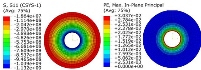
Fig. 19. (a) Hoop stress (b) Plasticity for 1200 MPa internal pressure
