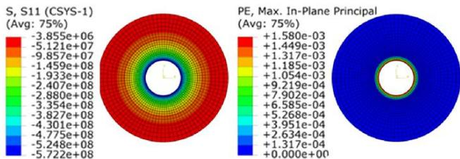
Fig. 16. (a) Hoop stress (b) Plasticity for 600 MPa internal pressure
