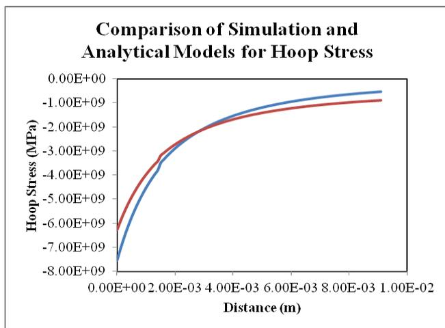
Fig. 24. Comparison of Analytical and Simulation Results for Hoop Stress along the radius of the cylinder
