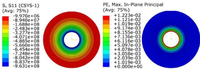
Fig. 18. (a) Hoop stress (b) Plasticity for 1000 MPa internal pressure
