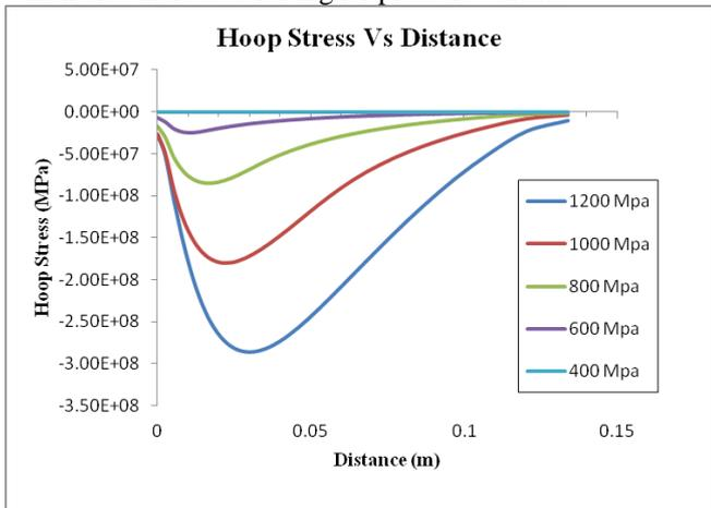
Fig. 20. Hoop Stress distribution along the radius of the cylinder against different internal pressures for no contact pressure steps
