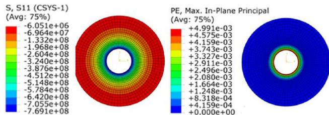
Fig. 10. a) Hoop stress (b) Plasticity for 800 MPa internal pressure
