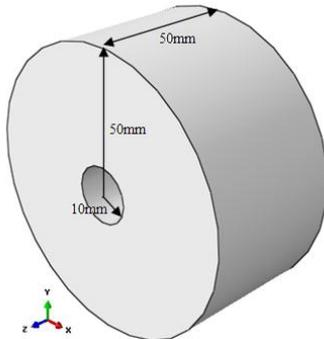
Fig. 2. Cross section of thick cylinder
