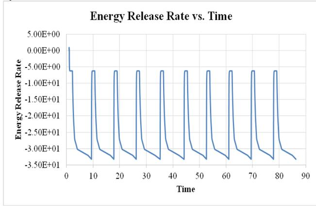
Fig. 23. Energy release rate vs. time for cyclic thermal loading on thick walled cylinder
