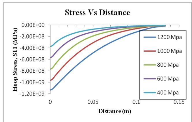
Fig. 13. Hoop Stress distribution along the radius of the cylinder against different internal pressures for Load Step
