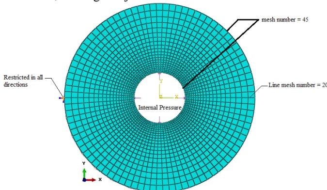
Fig. 3. Autofrettage model mesh and dimensions
