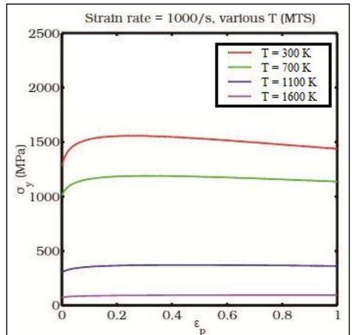
Fig. 5. Plastic properties of AISI 4340 SS at different temperatures[19]
