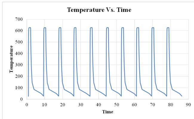
Fig. 22. Temperature vs. Time graph for thermally loaded thick walled cylinder
