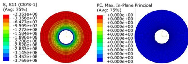
Fig. 8. (a) Hoop stress (b) Plasticity for 400 MPa internal pressure
