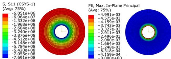
Fig. 17. (a) Hoop stress (b) Plasticity for 800 MPa internal pressure
