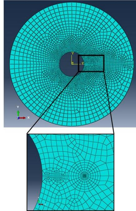
Fig. 6. Crack close-up showing meshed region around the crack tip
