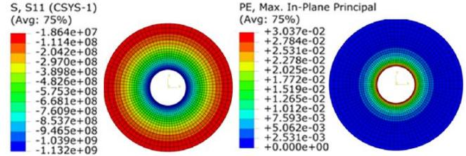
Fig. 12. (a) Hoop stress (b) Plasticity for 1200 MPa internal pressure
