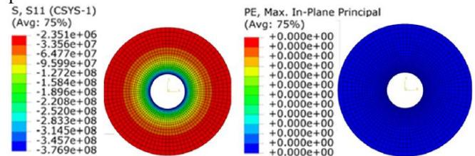
Fig. 15. (a) Hoop stress (b) Plasticity for 400 MPa internal pressure
