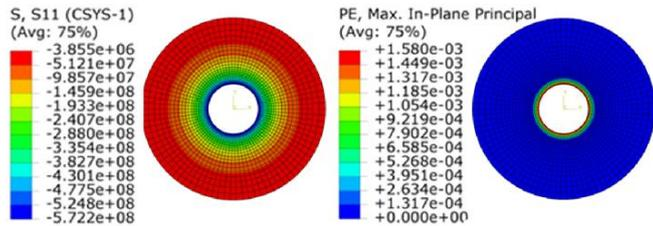
Fig. 9. a) Hoop stress (b) Plasticity for 600 MPa internal pressure
