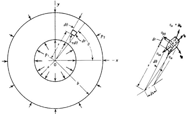
Fig. 1. Stress in thick walled cylinder[14]
