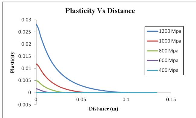
Fig. 21. Plasticity distribution along the radius of the cylinder against different internal pressures for no contact pressure steps
