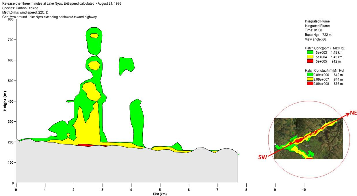
Fig. 12. Cross sectional view over lake (SW-NE) for entire 1 hour model run. Released gas is moving towards NE from SW direction following Terrain and moving parallel to the highway. Location of crosssectional view showing in figure inset.
