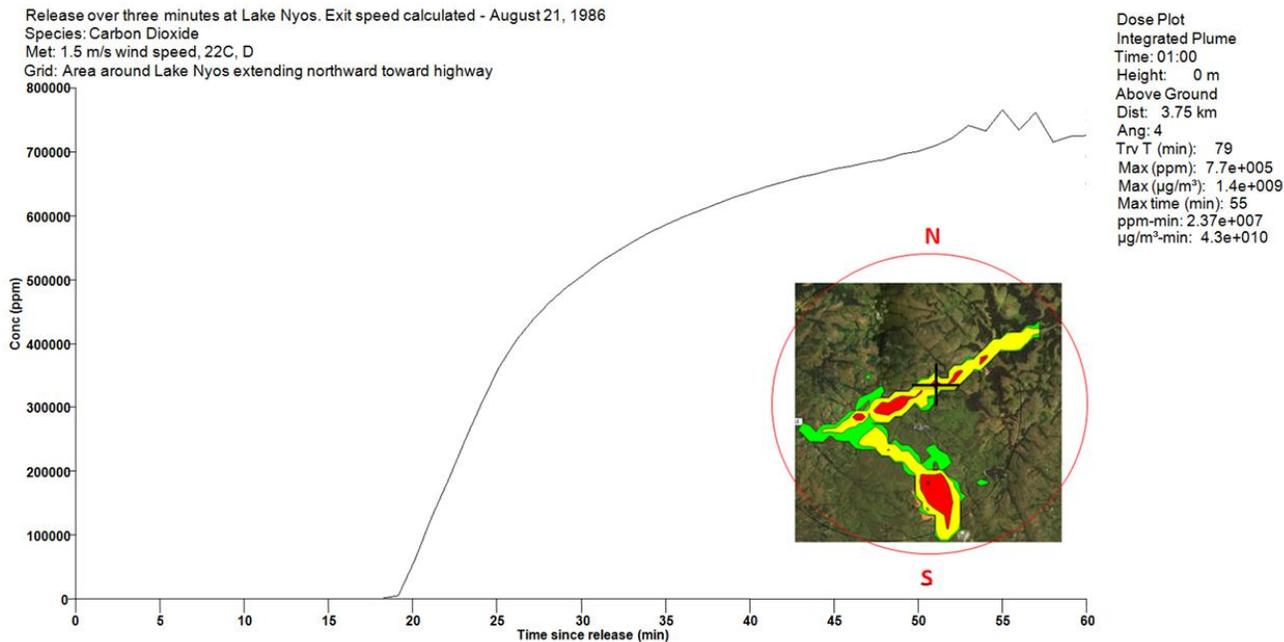
Fig. 13. Concentration in ppm versus Time in minute plot showing impact after release and reached at value around 800,000 ppm within 20 minutes. Location of selected location showing by “plus” in figure inset
