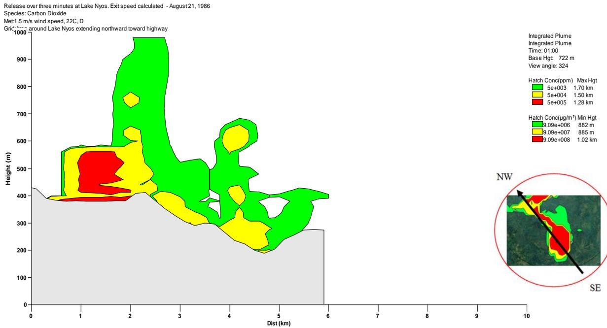
Fig. 11. Cross sectional view over lake (SE-NW) for entire 1 hour model run. Released gas is moving towards NW following Terrain. Location of crosssectional view showing in figure inset.
