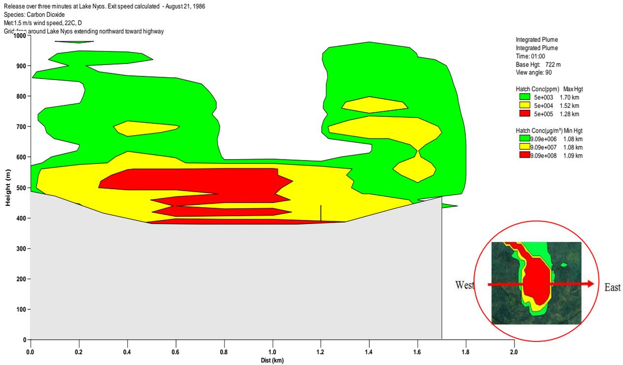
Fig. 10. Cross sectional view over lake (West-East) for entire 1 hour model run. Released gas is moving over hills present at both western and eastern side of Lake. Location of crosssectional view showing in figure inset.
