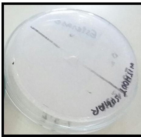
Fig. 11. Esterase activity on tween 80 agar plate in sugar starved suspension culture.
