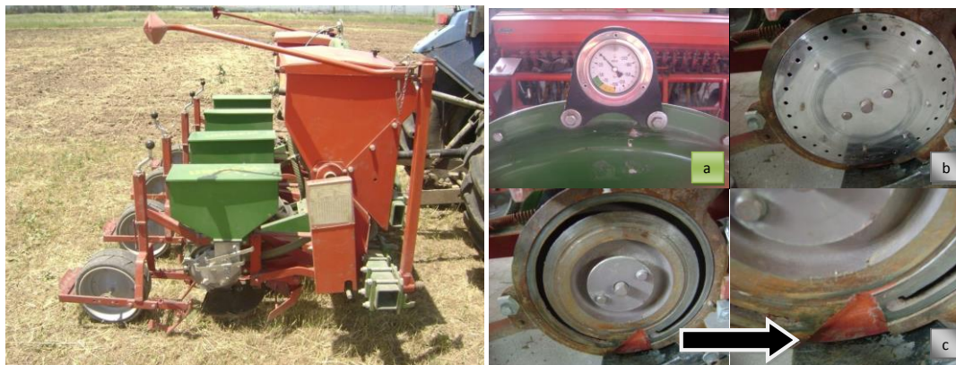
Figure 1. Pneumatic single seed planter. Vacuum meter (a), seed plate (b), and seed drop point (c)
