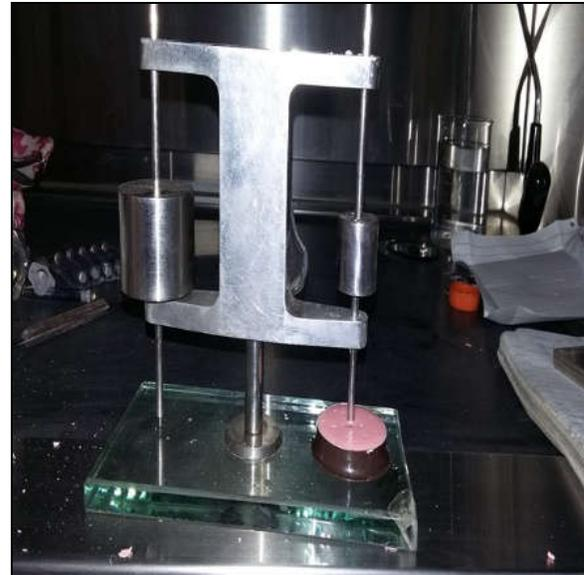
Figure-3: Setting time testing with Gillmore needle
