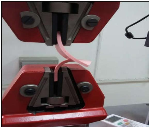
Figure-2: Tear strength testing with Universal Testing Machine
