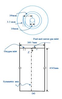
Figure 2a. Geometry of entrained flow gasifier
