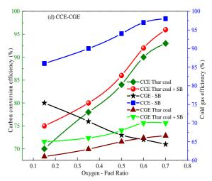
*Figure 5*.Effect of O/F ratio (a) Thar coal, (b) sugarcane bagasse (c) mixing of Thar coal and sugarcane bagasse (d) CCE & CGE
