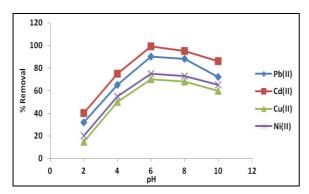
Figure 3. Adsorption of Pb(II), Cd(II), Cu(II) and Ni(II) by PMSAC at different pH values.
