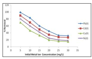
Figure 4. Adsorption of Pb(II), Cd(II), Cu(II) and Ni(II) by PMSAC at different initial metal ion concentrations
