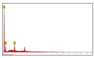
Figure 2. Energy Dispersive X-ray Spectrum of PMSAC
