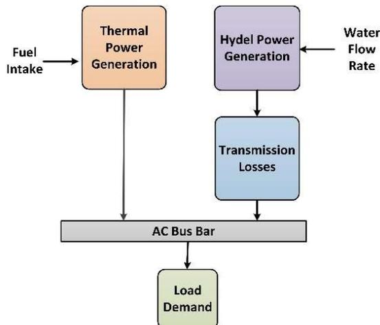
**Figure 1:** Hydro-thermal power generation system model
