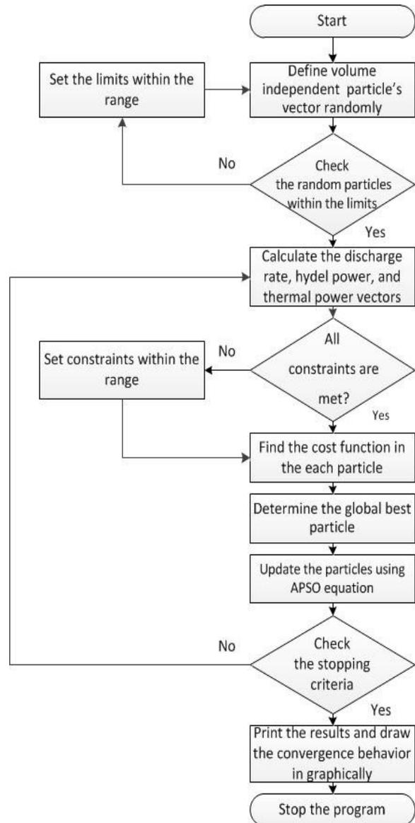
Figure 2: Flow chart of the proposed APSO algorithm.
