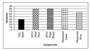
Figure 5. Comparison of hardness in the formulated compounds.
