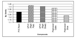
Figure 2. Comparison of Sp. Gravity in the formulated compounds.
