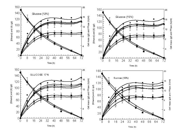
*Figure 2.* Effect of different glucose and sucrose concentrations (Glucose 12, 15 & 17%) and sucrose (15%) on ethanol formation ( $\circ$  : W; •: M), cell mass formed ( $\Delta$ : W;  $\blacktriangle$  : M), FFase ( $\diamond$ :W;  $\diamondsuit$ :M) formation and substrate present in fermentor ( $\Box$ :W; $\blacksquare$ : M) in batch culture at 40 °C. Error bars show standard error between mean of n = 3 observations.
