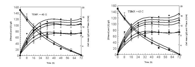
Figure 1. Effect of different Temperatures (40°C and 45°C) on ethanol formation ( $\circ$  : W; •: M), cell mass formed ( $\Delta$ : W; **A** : M), FFase ( $\diamond$ :W; •:M)formation and substrate present in fermentor ( $\Box$ :W; **a**: M) containing 15% sugars in molasses (pH 5.5).
