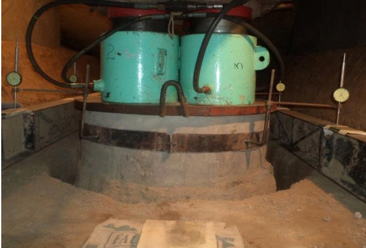
Fig. 4: A View of Jack, reference beams and the settlement gauges
