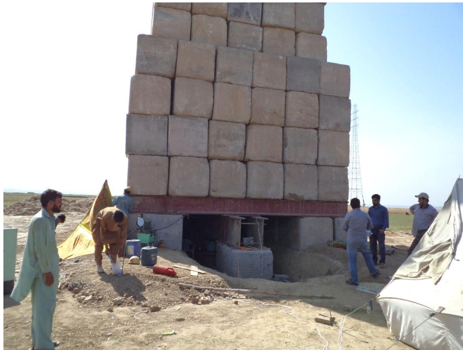
Fig. 3: Loading platform with concrete blocks
