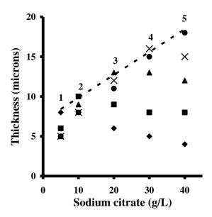
Figure 1: Effect of concentration of sodium citrate and sodium hypophosphite on thickness of electroless nickel plating from nickel chloride bath. Nickel chloride 10 g/L. 1-Sodium hypophosphite 5 g/L, 2- sodium hypophosphite 10 sodium g/L, 3hypophosphite 20 g/L, 4sodium hypophosphite 30 g/L
