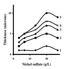
Figure 3: Effect of concentration of nickel sulfate on thickness of electroless nickel plating from nickel sulfate bath. 1- Sodium citrate/sodium hypophosphite 5/5 g/L, 2- Sodium citrate/sodium hypophosphite 10/10 g/L, 3-Sodium citrate/sodium hypophosphite 20/20 g/L, 4- Sodium citrate/sodium hypophosphite 30/30 g/L, 5- Sodium citrate/sodium hypophosphite 40/40 g/L
