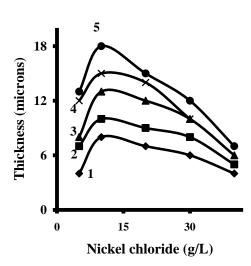
Figure 2: Effect of concentration of nickel chloride on thickness of electroless nickel plating from nickel chloride bath. 1-Sodium citrate/sodium hypophosphite 5/5 g/L, 2sodium citrate/sodium hypophosphite 10/10 g/L, sodium citrate/sodium 3hypophosphite 20/20 g/L, 4- sodium citrate/sodium hypophosphite 30/30 g/L, 5sodium citrate/sodium hypophosphite 40/40 g/L
