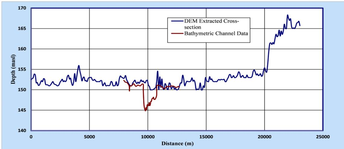
Fig. 8 Bathymetric data incorporation in DEM extracted cross-section
