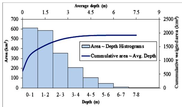
Fig. 20 Cumulative hypsometric curve and flooded area histograms
