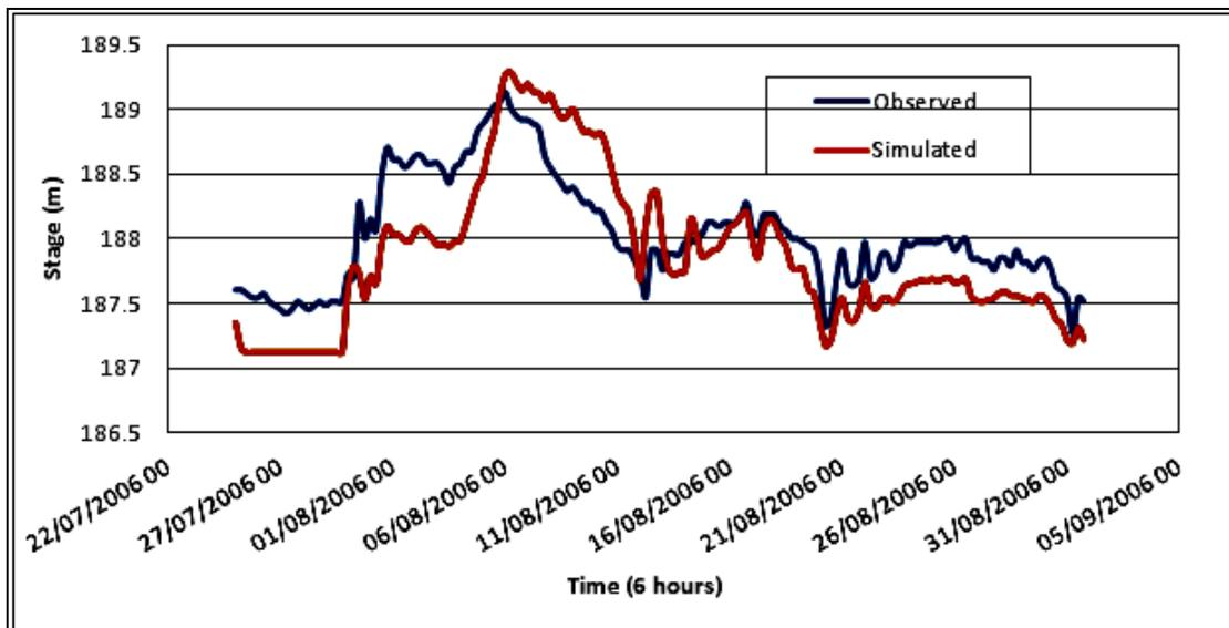
**Fig. 17:** Comparison of mode; stage hydrograph observed and simulated at Chashma, 2006 flood
