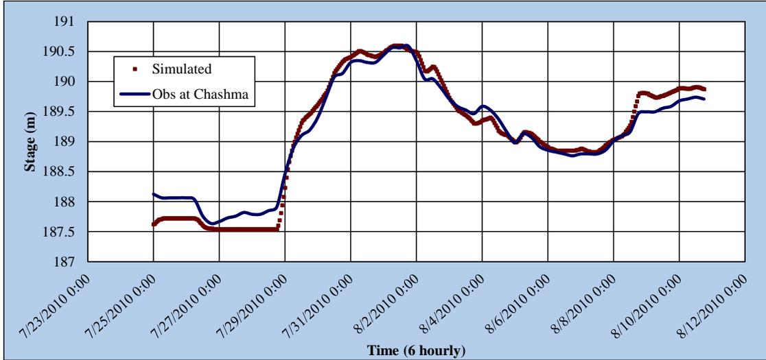
Fig. 14: Calibration of Model; Stage Hydrograph Observed and simulated at Chashma, 2010 flood
