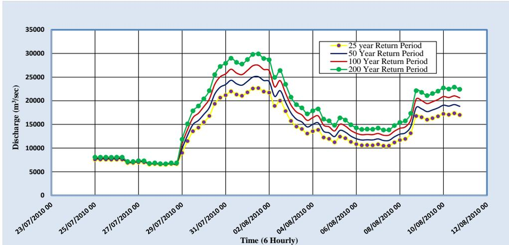
**Fig. 11** Frequency Distributions; Different Return Periods Flow Hydrograph at Chashma
