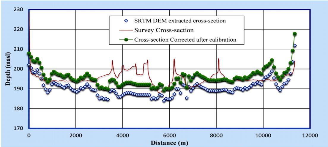
Fig. 7 Comparison of cross-sections; Corrected after calibration
