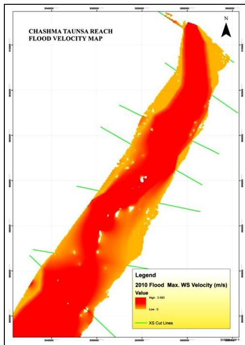
Fig. 21 A sample flood Velocity Map of Study Reach for 2010 Flood, d/s of Chashma (42 km Reach)
