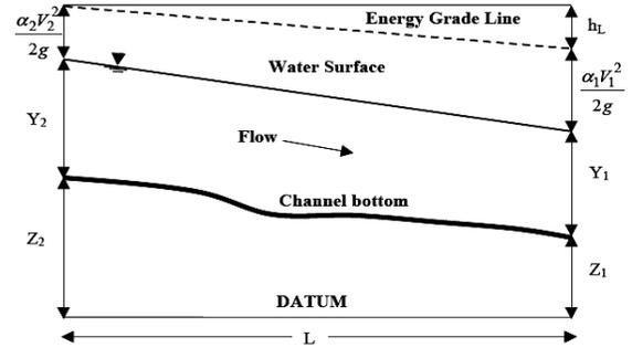
**Fig. 1** Energy equation parameters for gradually varied flow
