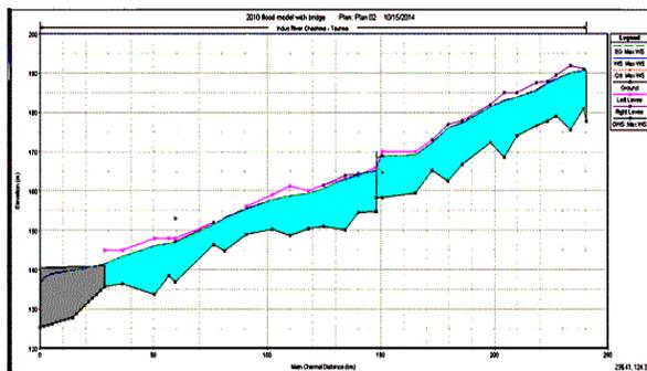
Fig. 13 Longitudinal profile of study reach for 2010 flood
