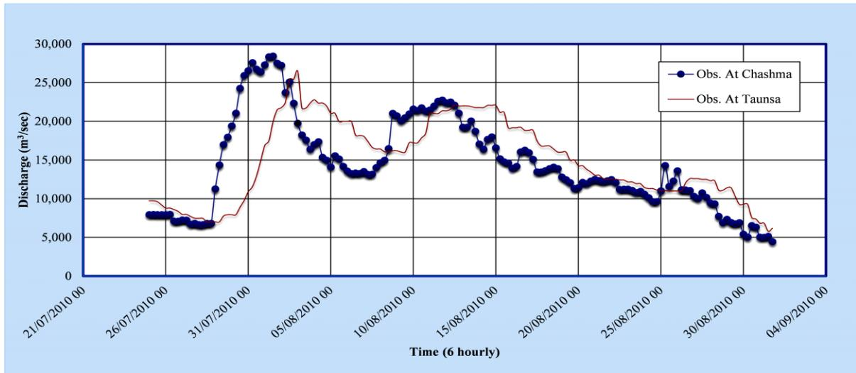
**Fig. 3** Observed flow hydrographs at Chashma and Taunsa of 2010 flood
