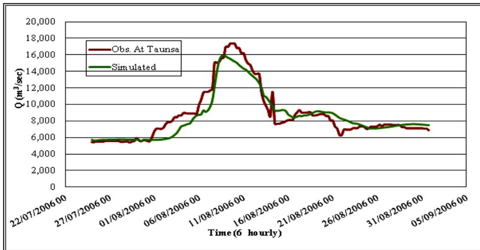
Fig. 16: Validation of model; flow Hydrograph; observed and simulated at Taunsa, 2006 flood
