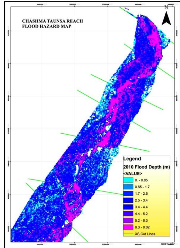
Fig. 22 A sample of flood Hazard Map of Study Reach for 2010 Flood d/s of Chashma (42km)
