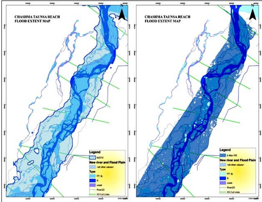
Fig. 18 Comparison of satellite and simulated flood extent for 2010 flood
