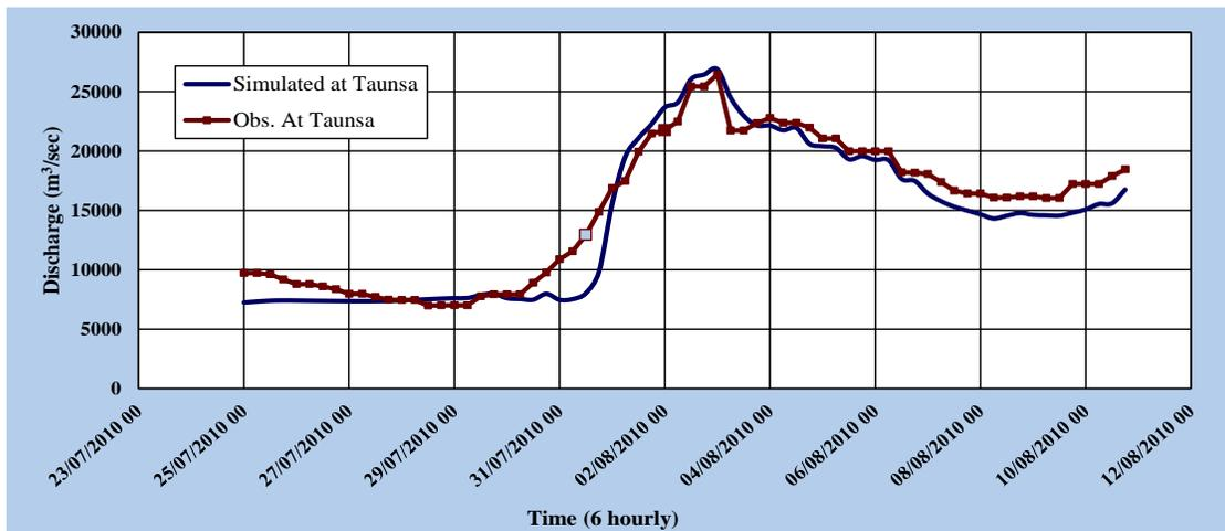
Fig. 15: Calibration of the model; Flow Hydrograph observed and simulated at Taunsa, 2010 flood
