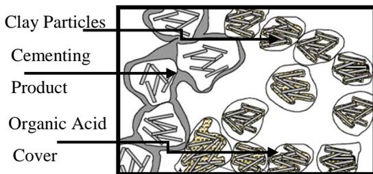
**Fig. 2** Clay particles with organic acid cover
