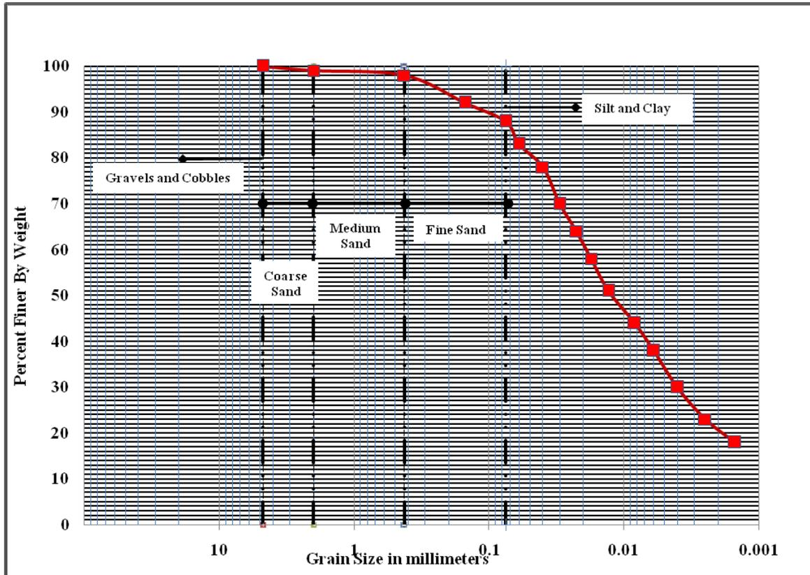
Fig. 6 Typical grain size distribution curve of mollisols
