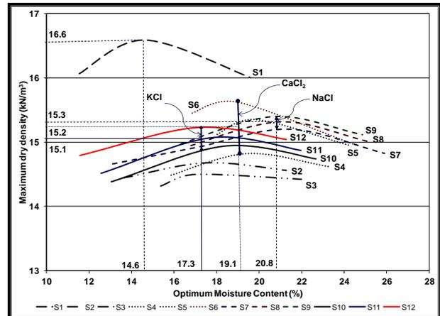
Fig. 8 Variation in modified proctor test characteristics of mollisols with addition of lime and salts
