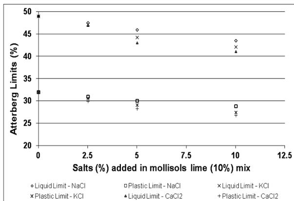
Fig. 7 Variation in Atterberg limits of mollisols lime mix by addition of salts
