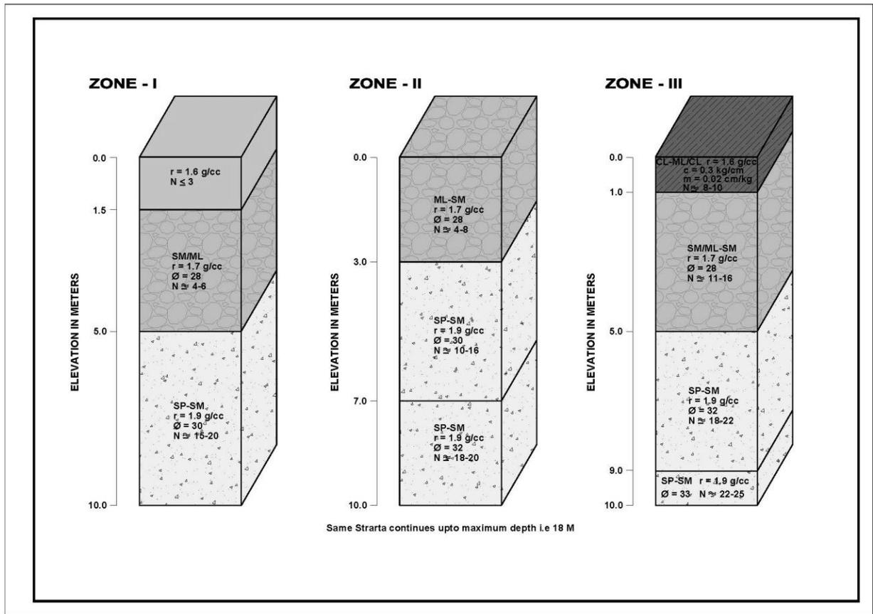
Fig. 6: General Stratification for Zone-I, II and III
