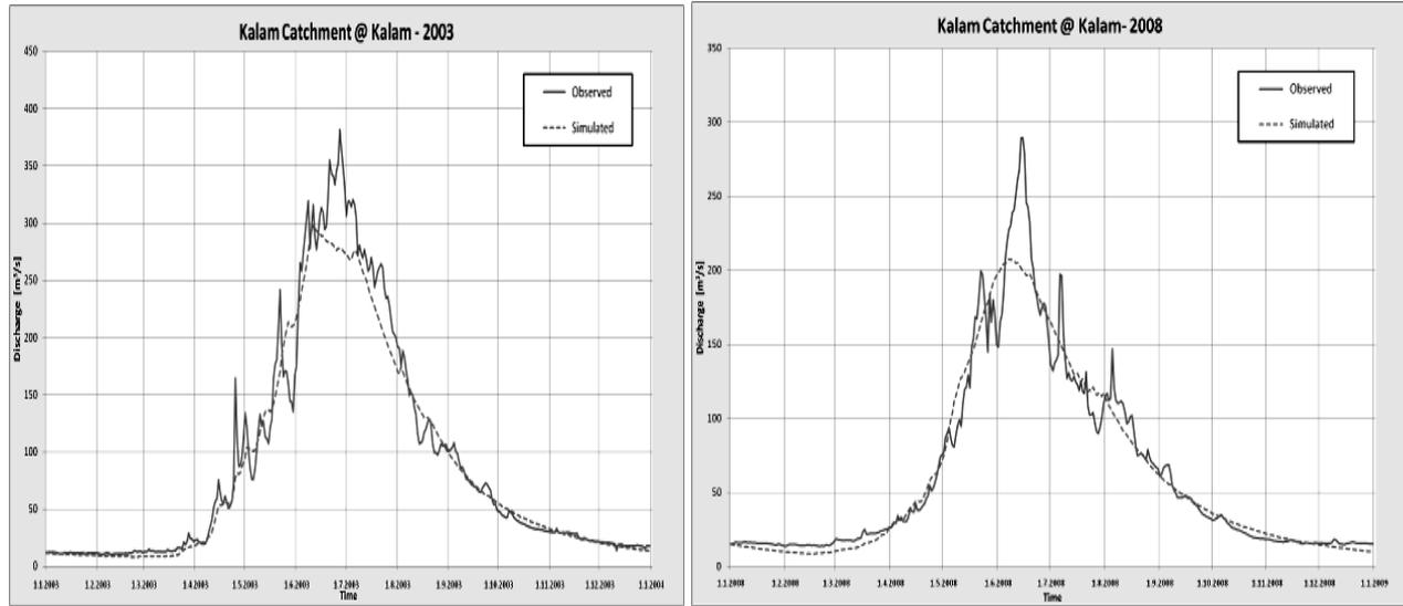
**Fig.14** Kalam one calibrating year 2003 and validating year 2008 (observed vs simulated) hydrograph
