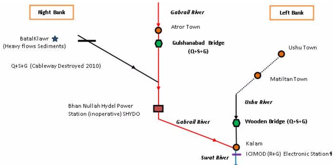
Fig. 3 Line diagram of River Swat catchment
