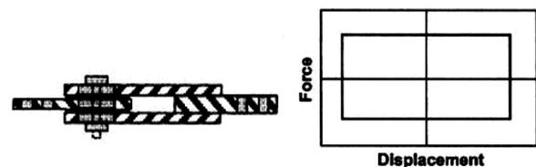
**Fig.5** Basic construction and idealized hysteresis behavior of friction damper
