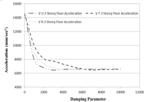
**Fig.45** Relation b/w Floor Acceleration & Damping Parameter (3-Storey Building)
