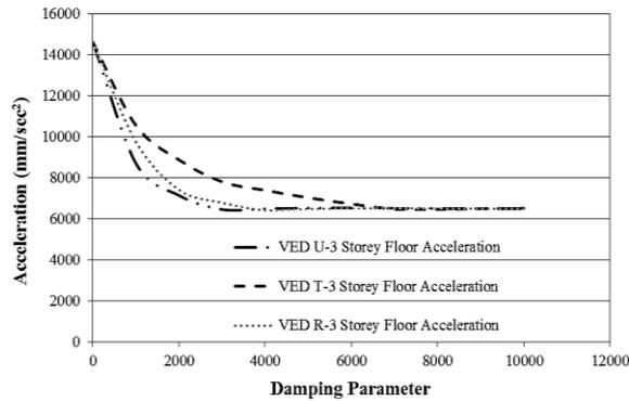
**Fig.48** Relation b/w Floor Acceleration & Damping Parameter (3-Storey Building)
