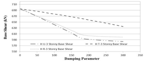
**Fig.27** Relation b/w Base Shear & Damping Parameter (3-Storey Building)
