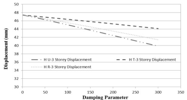
Fig.15 Relation b/w Displacement & Damping Parameter (3-Storey Building)
