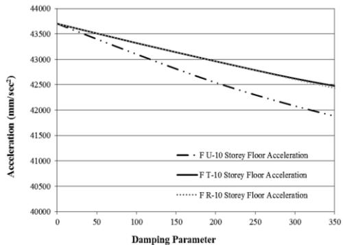
**Fig.44** Relation b/w Floor Acceleration & Damping Parameter (10-Storey Building)
