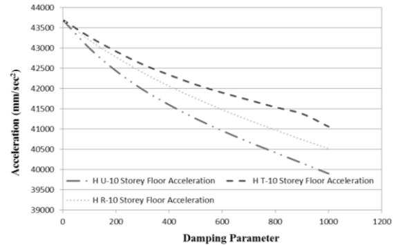
Fig.41 Relation between Floor Acceleration and Damping Parameter (10-Storey Building)
