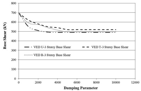
**Fig.36** Relation b/w Base Shear & Damping Parameter (3-Storey Building)
