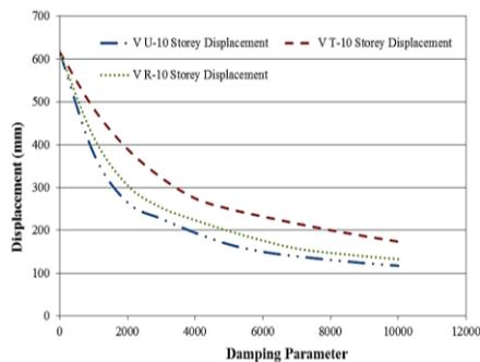
**Fig.23** Relation b/w Displacement & Damping Parameter (10-Storey Building)
