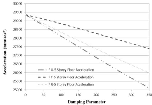
**Fig.43** Relation b/w Floor Acceleration & Damping Parameter (5-Storey Building)
