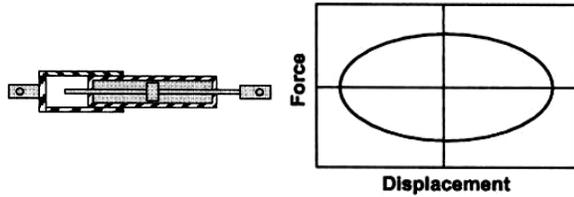
**Fig.7** Basic construction and idealized hysteresis behavior of viscous damper
