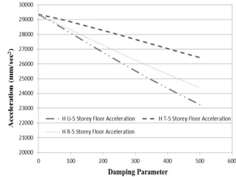
Fig.40 Relation b/w Floor Acceleration & Damping Parameter (5-Storey Building)
