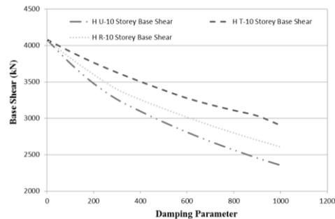
**Fig.29** Relation b/w Base Shear & Damping Parameter (10-Storey Building)
