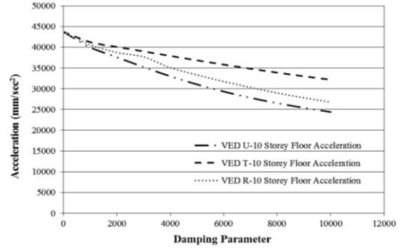
**Fig.50** Relation b/w Floor Acceleration & Damping Parameter (10-Storey Building)
