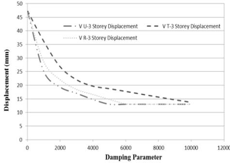
**Fig.21** Relation b/w Displacement & Damping Parameter (3-Storey Building)
