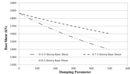
**Fig.28** Relation b/w Base Shear & Damping Parameter (5-Storey Building)
