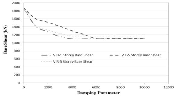
**Fig.34** Relation b/w Base Shear & Damping Parameter (5-Storey Building)
