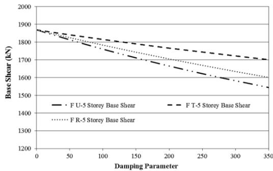
**Fig.31** Relation b/w Base Shear & Damping Parameter (5-Storey Building)
