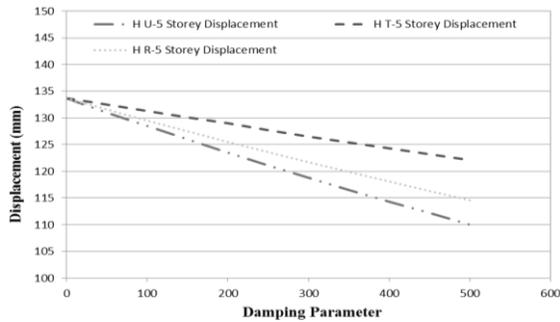
**Fig.16** Relation b/w Displacement & Damping Parameter (5-Storey Building)
