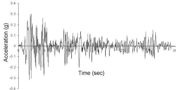
**Fig.10** E-W Direction Time Acceleration Graph of El-Centro Earthquake
