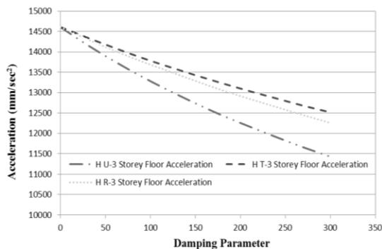
Fig.39 Relation b/w Floor Acceleration & Damping Parameter (3-Storey Building)
