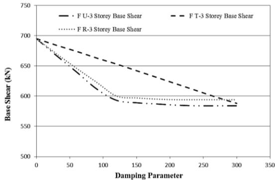
**Fig.30** Relation b/w Base Shear & Damping Parameter (3-Storey Building)
