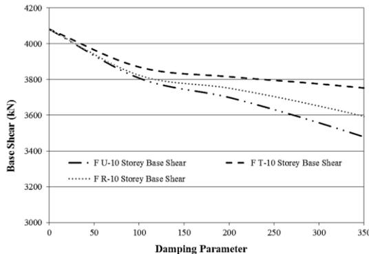
**Fig.32** Relation b/w Base Shear & Damping Parameter (10-Storey Building)
