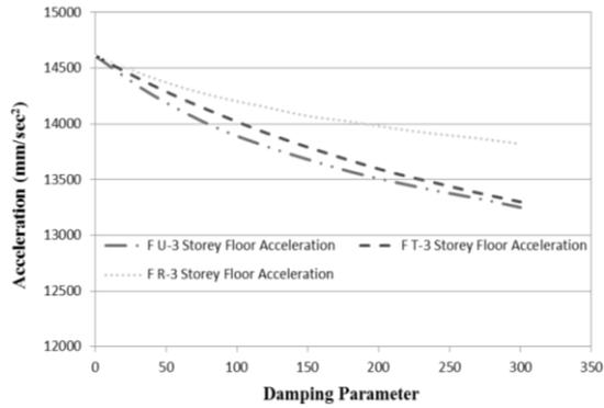
**Fig.42** Relation b/w Floor Acceleration & Damping Parameter (3-Storey Building)
