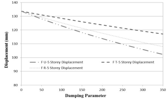
**Fig.19** Relation b/w Displacement & Damping Parameter (5-Storey Building)
