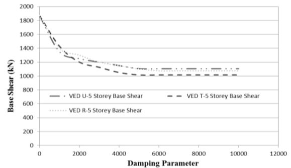
**Fig.37** Relation b/w Base Shear & Damping Parameter (5-Storey Building)
