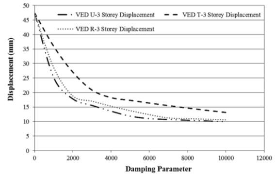
**Fig.24** Relation b/w Displacement & Damping Parameter (3-Storey Building)
