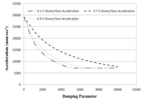
**Fig.46** Relation b/w Floor Acceleration & Damping Parameter (5-Storey Building)
