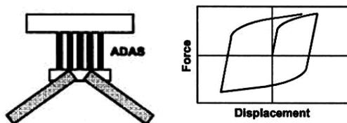
**Fig.3** Basic construction and idealized hysteresis behavior of Hysteretic damper
