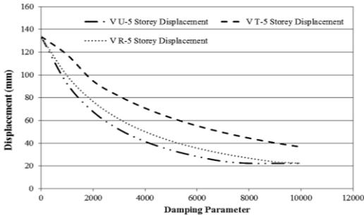
**Fig.22** Relation b/w Displacement & Damping Parameter (5-Storey Building)
