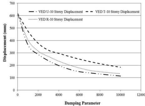
**Fig.26** Relation b/w Displacement & Damping Parameter (10-Storey Building)
