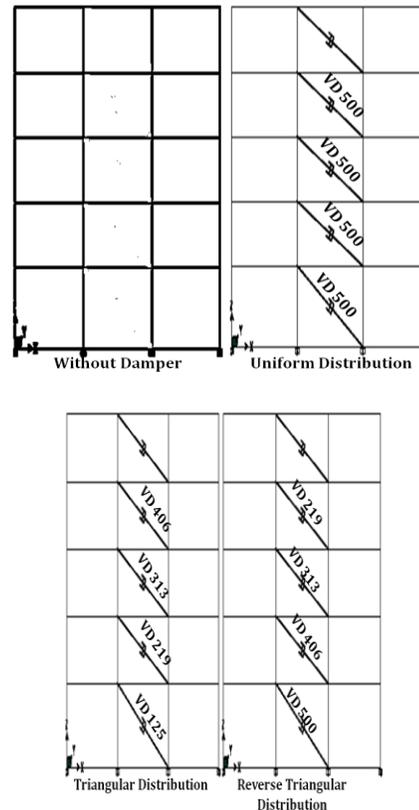
**Fig.12** Damper Distribution with Height
