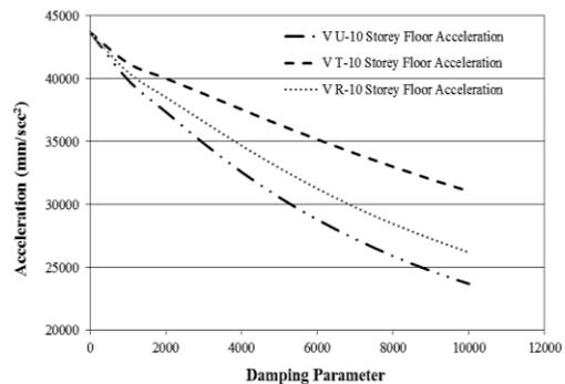
**Fig.47** Relation b/w Floor Acceleration & Damping Parameter (10-Storey Building)
