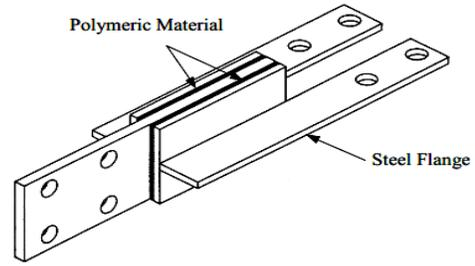
**Fig.8** Visco-elastic damper [7]
