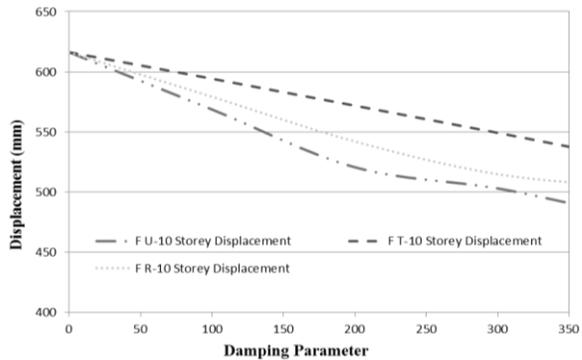
**Fig.20** Relation b/w Displacement & Damping Parameter (10-Storey Building)
