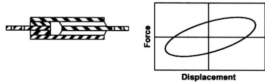
**Fig.9** Basic construction and idealized hysteresis behavior of visco-elastic damper
