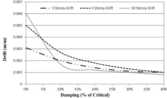
Fig.13 Relation b/w Drift & Increasing Damping Ratio
