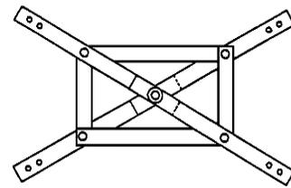
**Fig.4** Pall Friction Damper [10]
