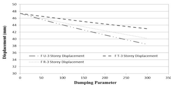
**Fig.18** Relation b/w Displacement & Damping Parameter (3-Storey Building)
