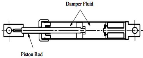
**Fig.6** Viscous fluid damper [14]
