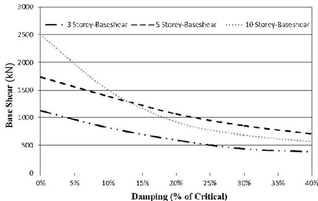
Fig.14 Relation b/w Base Shear & Increasing Damping Ratio
