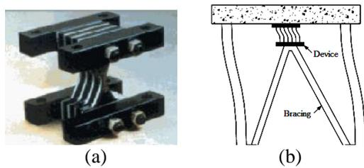
**Fig.2** (a) Added Damping and stiffness (ADAS) Damper (b) Idealized building structure with supplemental yielding Hysteretic element. [7]
