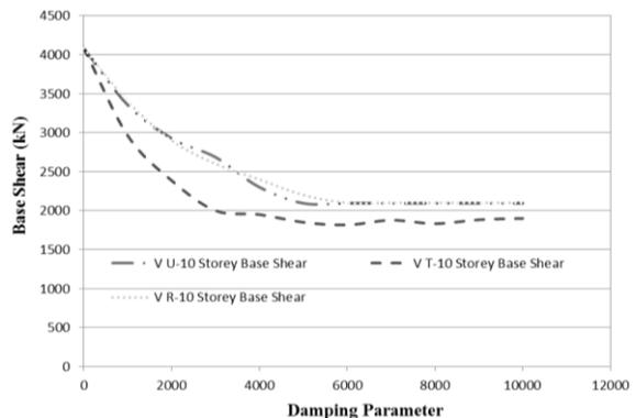
**Fig.38** Relation b/w Base Shear & Damping Parameter (10-Storey Building)
