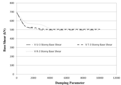
**Fig.33** Relation b/w Base Shear & Damping Parameter (3-Storey Building)
