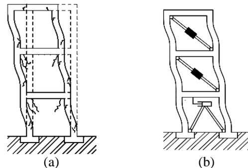
**Fig.1** (a) Conventional design of seismic resistant structure (b) Structure with passive dissipation devices
