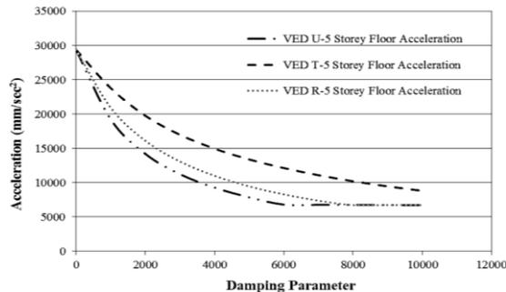
**Fig.49** Relation b/w Floor Acceleration & Damping Parameter (5-Storey Building)
