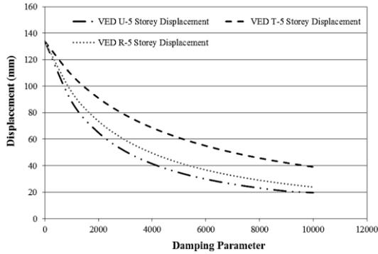
**Fig.25** Relation b/w Displacement & Damping Parameter (5-Storey Building)
