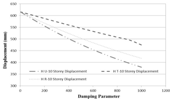
**Fig.17** Relation b/w Displacement & Damping Parameter (10-Storey Building)
