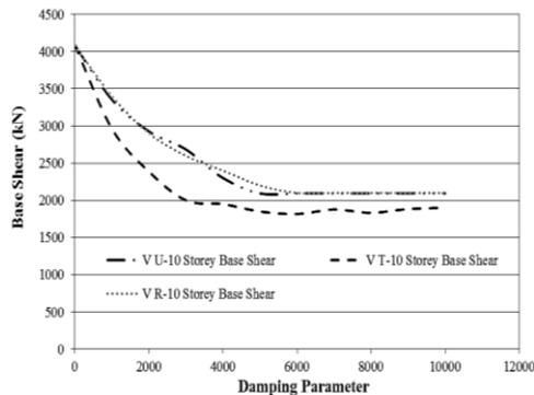
**Fig.35** Relation b/w Base Shear & Damping Parameter (10-Storey Building)
