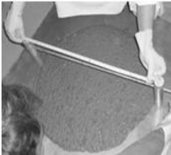
Fig.10 Slump flow test (ASTM-C1611/C1611M)
