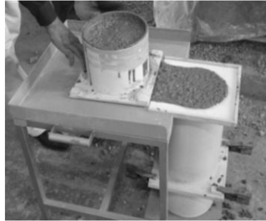
Fig.12 Static stability test (ASTM C1610 /C1610M)
