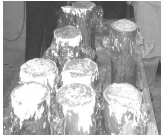
Fig.13 Capped Concrete filled cylinders for compressive strength tests
