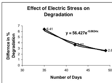
**Fig. 3** Degradation under electric stress.
