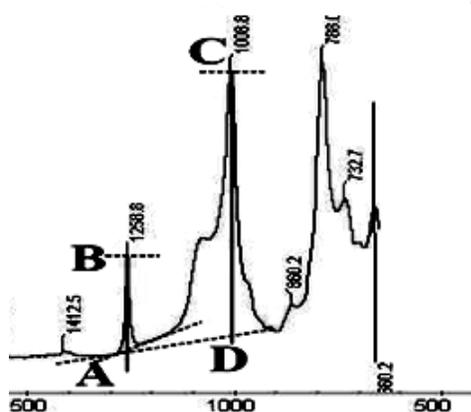
**Fig 2.** Analysis of aging of polymeric insulators using FTIR spectroscopic technique Change of absorption peak ratio -  $\frac{APR_{TS} - APR_{OS}}{APR_{OS}}$
