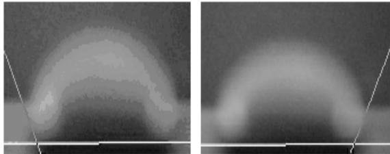
(c) B2 (0.32mg/cm<sup>2</sup>) Angle 65°, Angle 64°, Contact angle 115.5°
