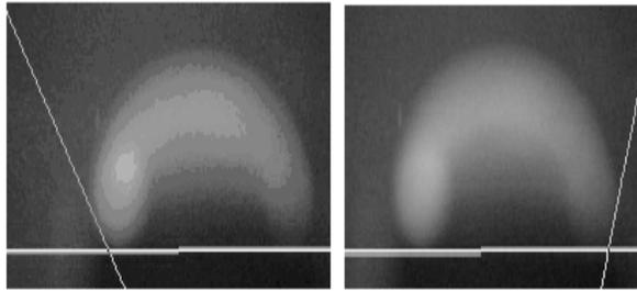
(b) B1 (0.31mg/cm<sup>2</sup>) Angle 55° Angle 73°, contact angle 116°
