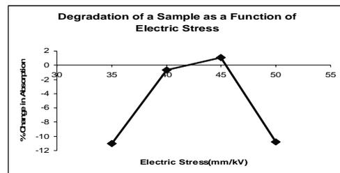
**Fig.5.** Sample degradation as a function of electric stress
