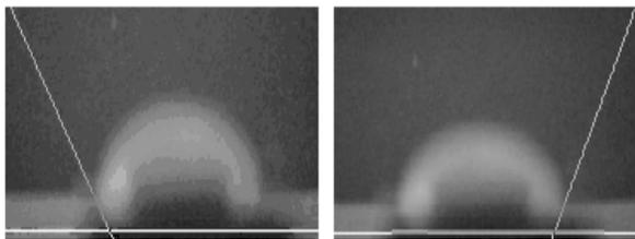
(a) B4 (1.29mg/cm<sup>2</sup>) Angle 61° Angle 65°, Contact angle 117°
