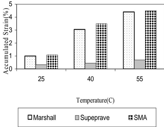
**Fig. 6** Accumulated stains of the mixes versus temperature At 500 kPa
