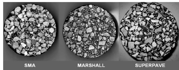
**Fig.1** Structural comparison of SMA, MARSHALL and SUPERPAVE
