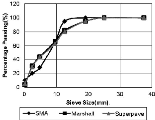
Fig. 2 Design Aggregate Gradation
