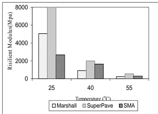
Fig.11 Resilient Modulus Vs Temperature
