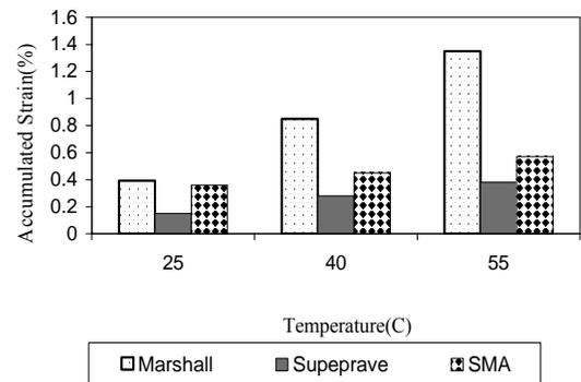
Fig.4 Accumulated stains of the mixes versus temperature at 100 kPa
