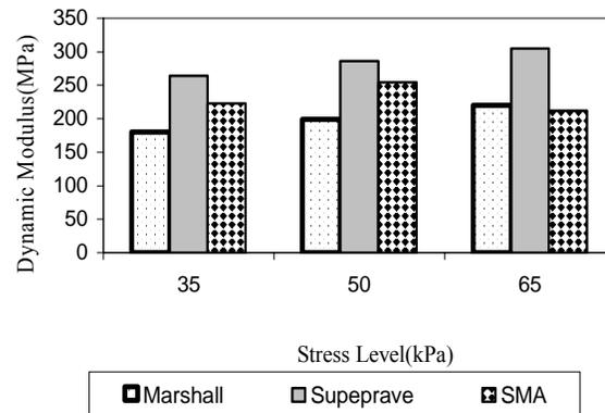
**Fig.10** Dynamic modulus versus stress Levels at 55°C
