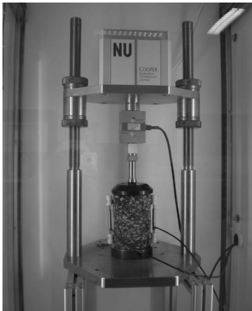
**Fig.7** Dynamic modulus testing arrangement using NU-14
