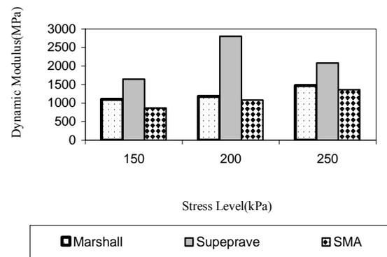
**Fig.9** Dynamic modulus versus stress Levels at 40°C
