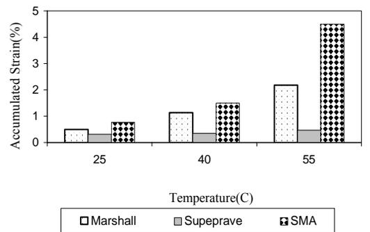
Fig. 5 Accumulated stains of the mixes versus temperature at 300 kPa
