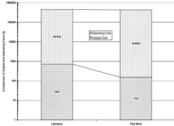
**Fig. 8:** Comparison of capital and operating cost (pumping + exergy destruction cost)
