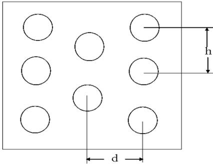
Fig. 2: Side view of heat exchanger to show tube arrangement
