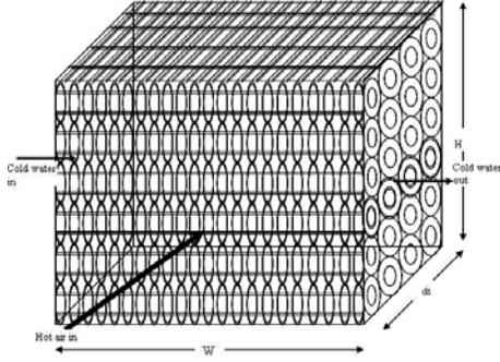
Fig. 1: A view of annular fin heat exchanger
