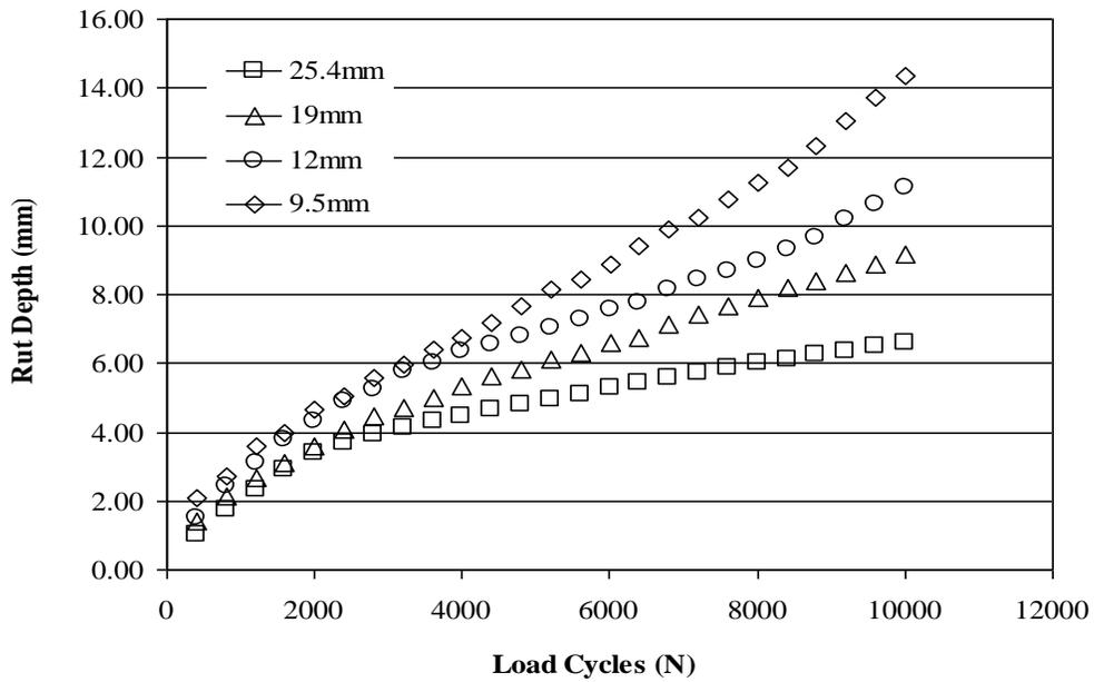
Fig.4c Influence of load cycles on rut depth at 60°C
