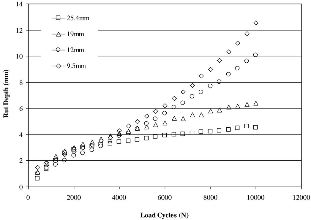
Fig.4b Influence of load cycles on rut depth at 40°C
