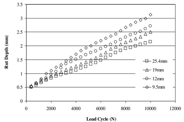
**Fig.4a** Influence of load cycles on rut depth at  $25^{\circ}\text{C}$
