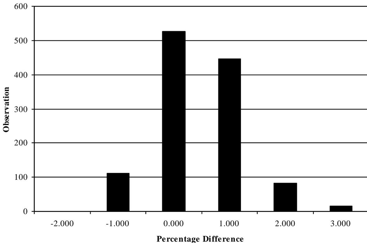
Fig. 7 Percentage Differences between the observed and the predicted rut depth.
