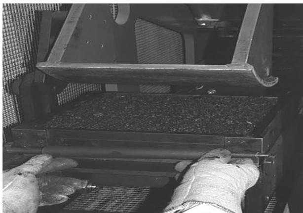
**Fig. 2** Slab specimen preparations on Roller Compactor [12]
