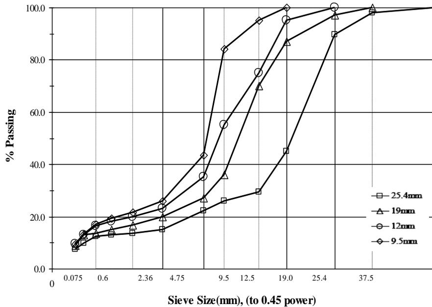
**Fig.1** Selected Aggregate Gradations for SMA Mixtures
