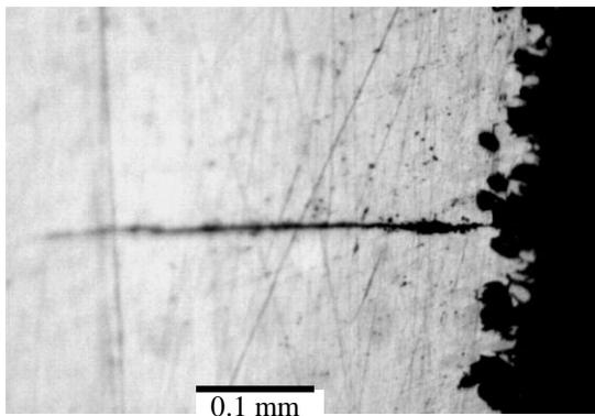
**Figure 4:** Optical Micrograph showing one of the four cracks in Blade # 2. The narrowness of the crack as it approaches the surface suggests that the crack had essentially formed beneath the surface.
