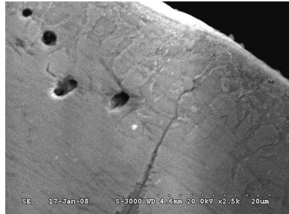
**Figure 5:** Scanning Electron Micrograph of the same crack shown in Figure 4. It is interesting to note in this micrograph that the coating does not exhibit any cracking at this stage.
