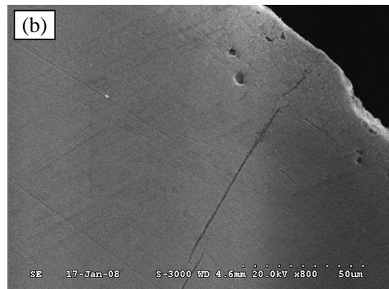
**Figure 6:** (a & b): Optical and Scanning Electron Micrographs taken from another location of Blade # 2, illustrating that the cracks are not exposed to surface, and hence cannot be related to corrosion fatigue. It may also be noted that in addition to the small crack just beneath the surface, there are two more independent sub-surface cracks.
