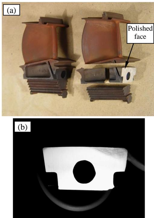
**Figure 1:** (a & b): Photograph illustrating the manner in which the Turbine Blades were sectioned for metallographic examination.
