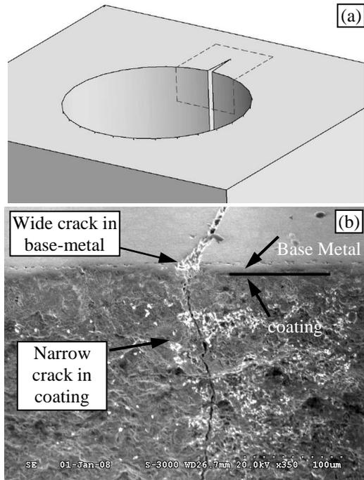
**Figure 3:** Scanning-Electron-Micrograph taken by tilting the specimen in such a manner that both the metallographically-polished surface as well as a part of the inside surface of the air-inlet hole could be seen. The scanned portion of the two surfaces which were essentially at right angle to each other are schematically illustrated in Figure 3a.
