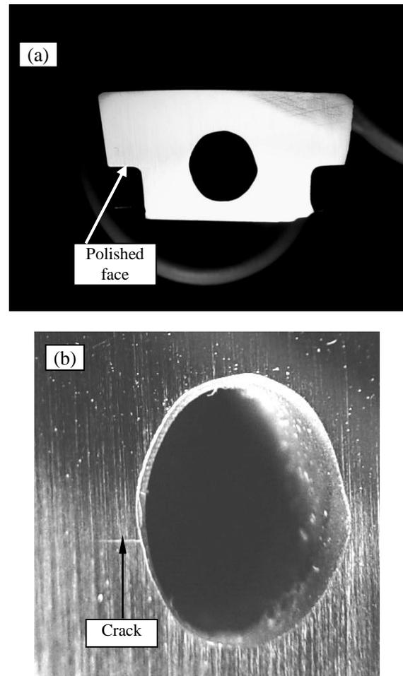
**Figure 2:** (a & b): Photograph showing the location and orientation of cracks in Blade # 1. The crack became visible to naked eye even before the final stage of polishing.
