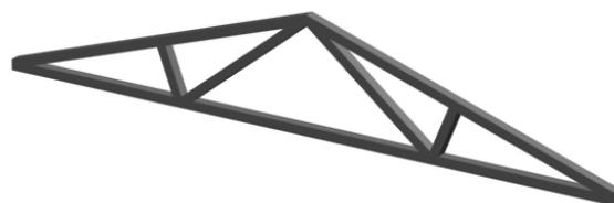
**Figure 10:** Truss used for roofing system.
