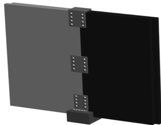
**Figure 7:** Panels with bolted connection details
