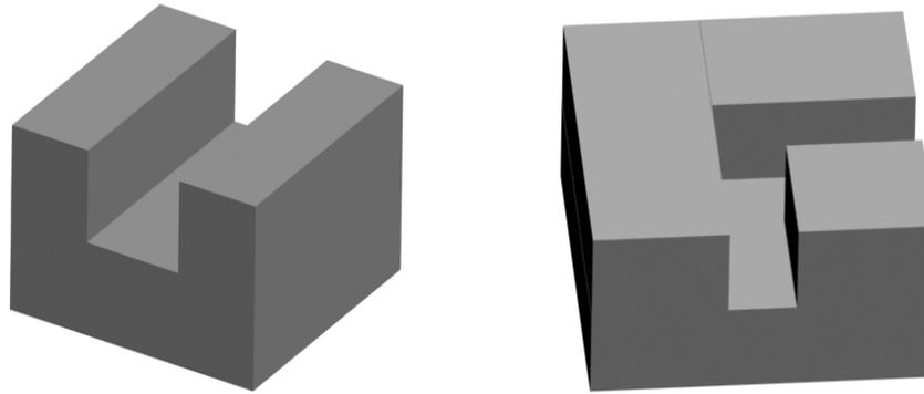
**Figure 12:** Side and corner foundation blocks
