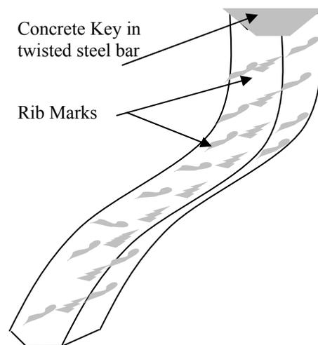
Figure 1: Concrete Key in twisted steel bar [2]
