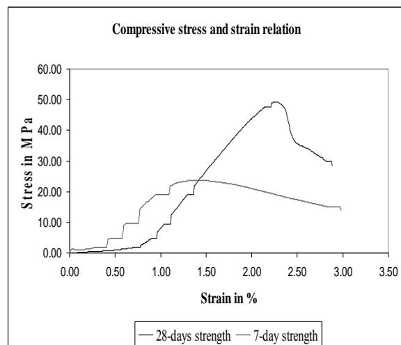
Figure 6: Compressive strengths of concrete
