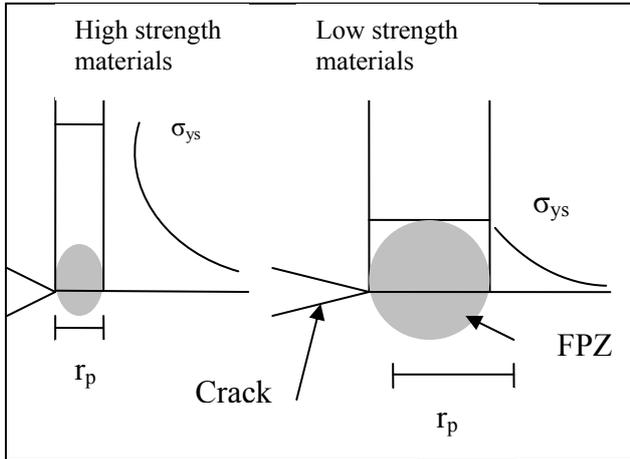
**Figure 2:** Fracture process zone in HSC and NSC [15]
