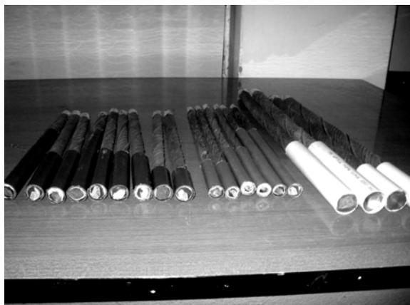
Figure 4: Steel bars for pullout test
