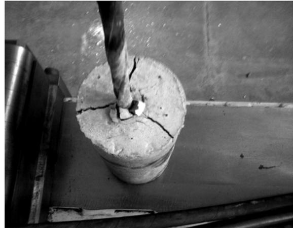
Figure 9: Longitudinal splitting cracks
