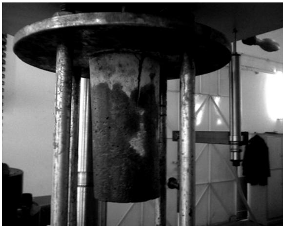
Figure 8: Pull out test in UTM
