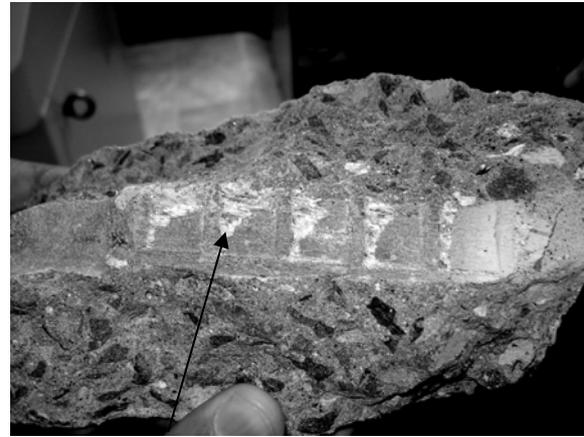
**Figure 3:** Wedges due to crushing of concrete
