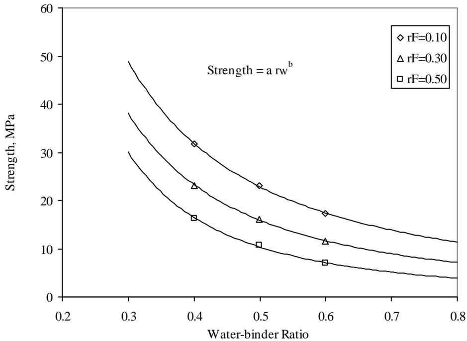
Figure 1: Strength vs Water-binder ratio plots with power fits
