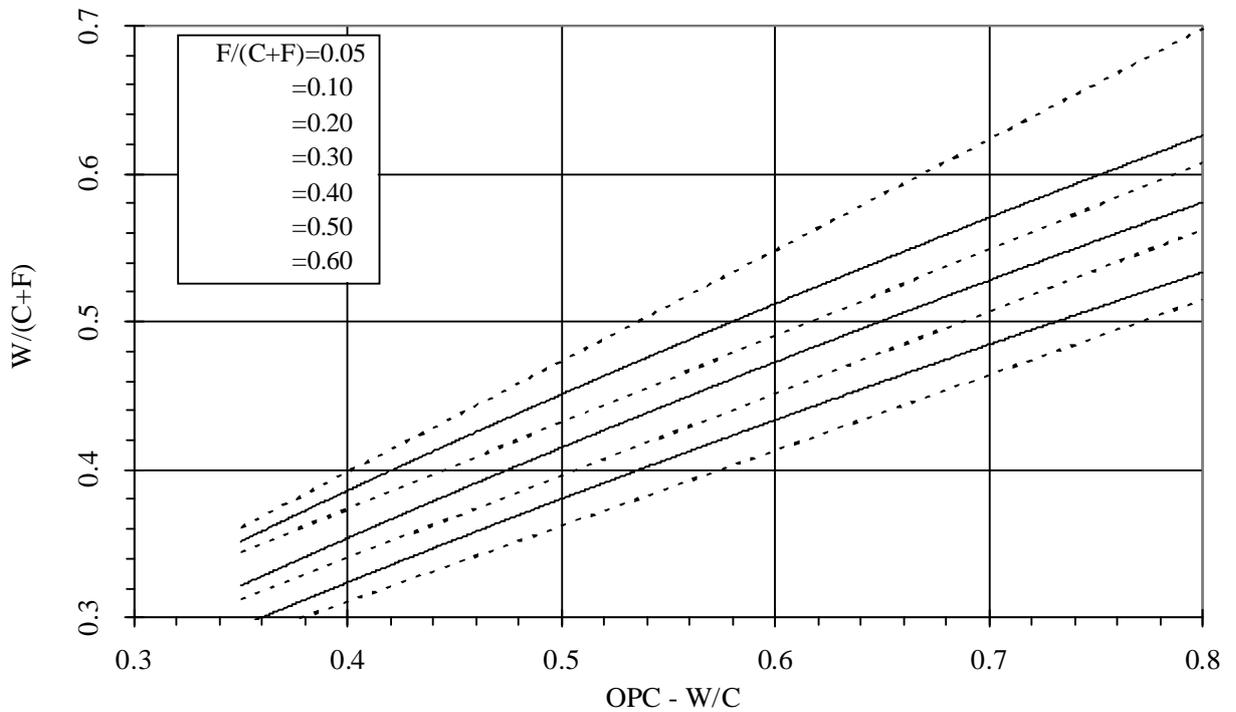
Figure 5: Water-modification chart for high calcium fly ash
