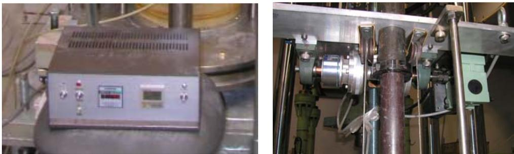
**Figure 8:** (a) Counter used to count number of blows and (b) Pulley, motor and clutch system to lift the hammer for free fall.
