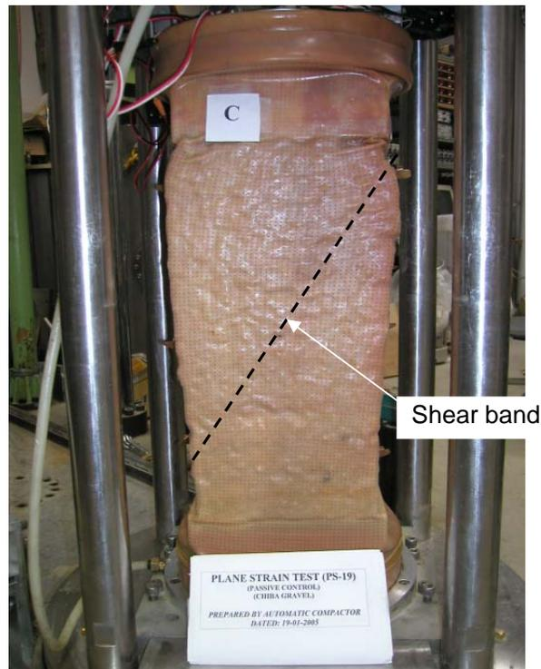
Figure 25: Shear band formation in PS-19 with dry density of  $2.02 \text{ g/cm}^3$ .
